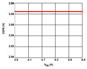
FIGURE 9. V2P8 OUTPUT vs INPUT VOLTAGE
