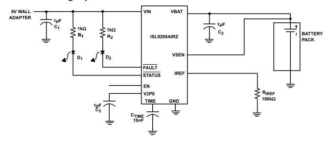
FIGURE 2. TYPICAL APPLICATION: 3x3 DFN PACKAGE OPTION
