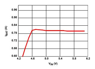
FIGURE 8. CHARGE CURRENT vs INPUT VOLTAGE
