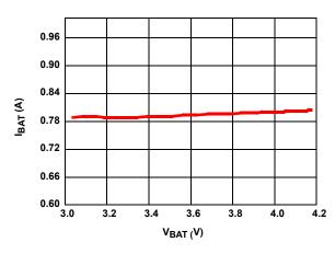
FIGURE 6. CHARGE CURRENT vs OUTPUT VOLTAGE
