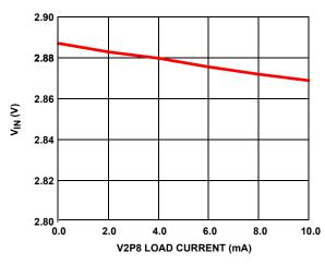
FIGURE 10. V2P8 OUTPUT vs ITS LOAD CURRENT
