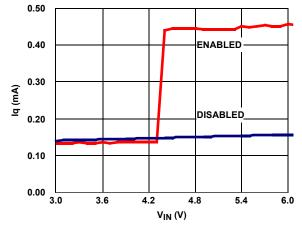
FIGURE 13. INPUT QUIESCENT CURRENT vs INPUT VOLTAGE
