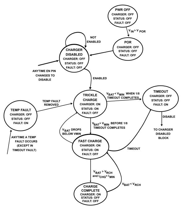
FIGURE 17. STATE MACHINE DIAGRAM
