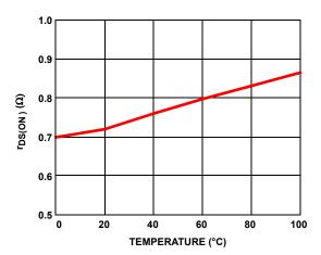
FIGURE 11.  $r_{DS(ON)}$  vs TEMPERATURE AT 3.7V OUTPUT
