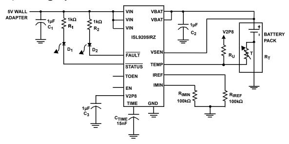
FIGURE 1. TYPICAL APPLICATION: 3x3 QFN PACKAGE OPTION
