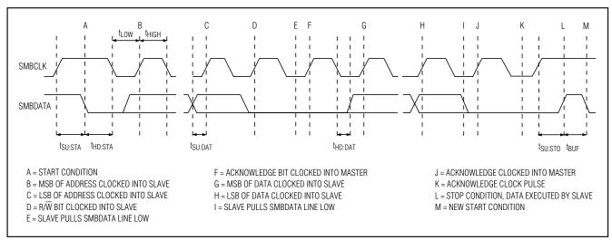
Figure 4. SMBus Write Timing Diagram
