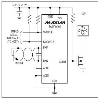
Figure 3. Fan Control Application
