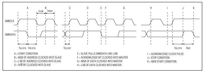
Figure 5. SMBus Read Timing Diagram
