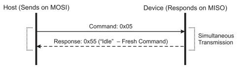
Figure 4-2. Sleep Command – CRC Enabled
