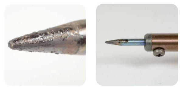
If after cleaning on the sponge / brass shavings the tip is still not shiny then melt a small amount of solder onto it and clean again. The flux in the solder will help to clean the tip.
