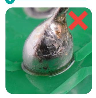
Too much solder on a joint can cause bridging to adjacent components, leading to a short circuit.
