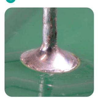
This photo shows an *ideal* solder joint: there is enough solder to form a nice fillet, without excessive solder bulging out. The component leg is ideally in the centre of the joint.
