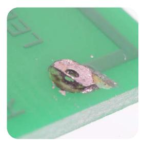
If a PCB is overheated the most likely outcome is that the copper layer will delaminate from the fibre glass board. This usually leads to broken joints and a non-working circuit.
