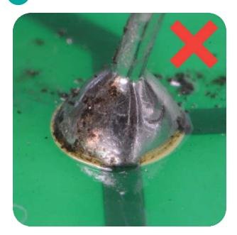
The PCB tracks are covered in a special paint called solder resist. This helps prevent the solder from flowing away from the joint. As more solder is added it builds into a blob, as shown in the next 2 photos:
