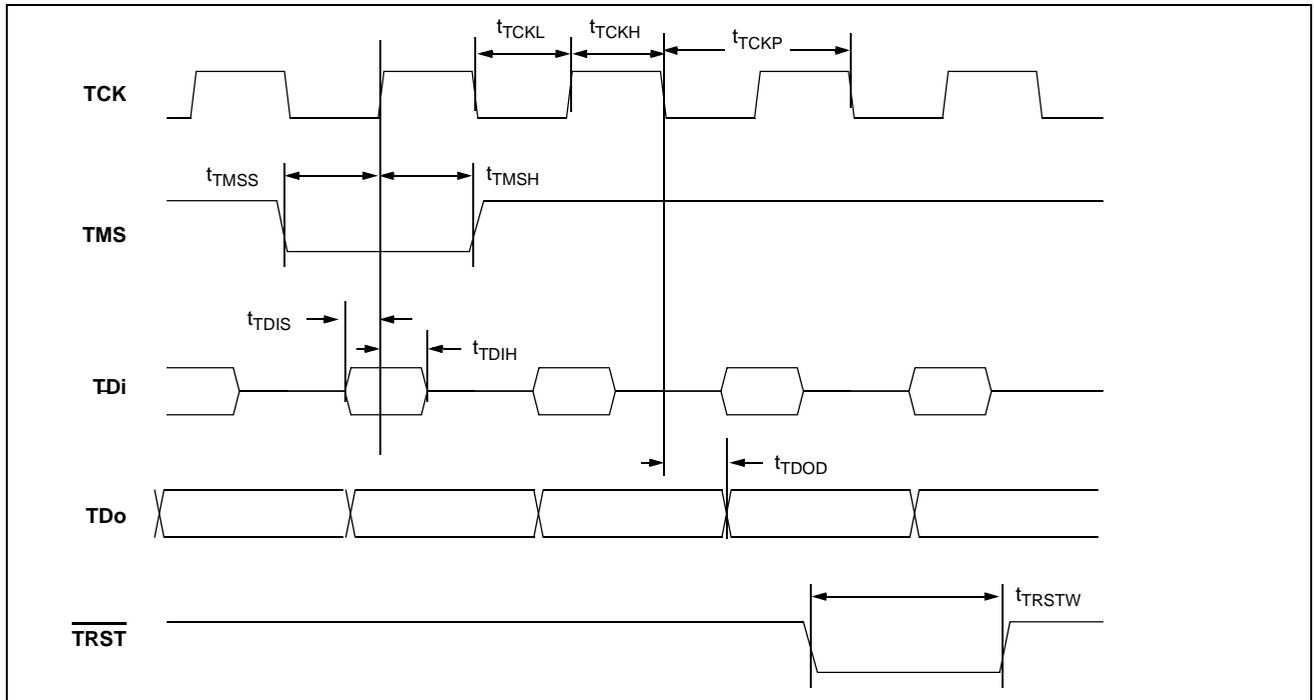
**Figure 27 - JTAG Test Port Timing Diagram**
