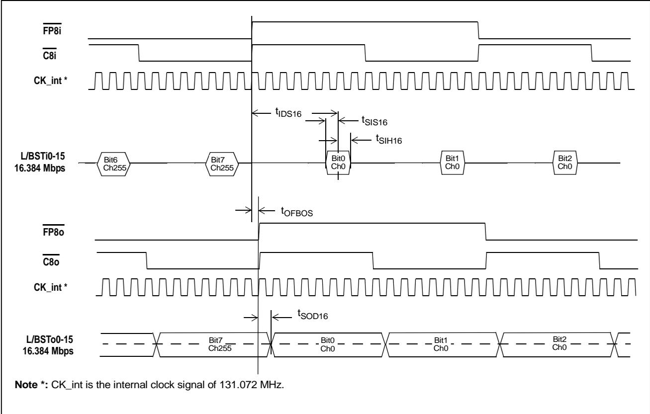
Figure 23 - GCI-Bus Local/Backplane Data Timing Diagram (16 Mbps)
