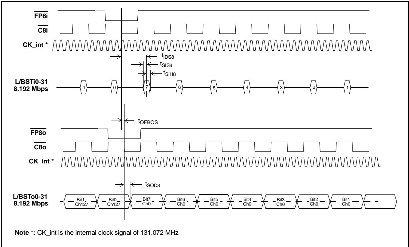
Figure 20 - ST-BUS Local/Backplane Data Timing Diagram (8 Mbps)
