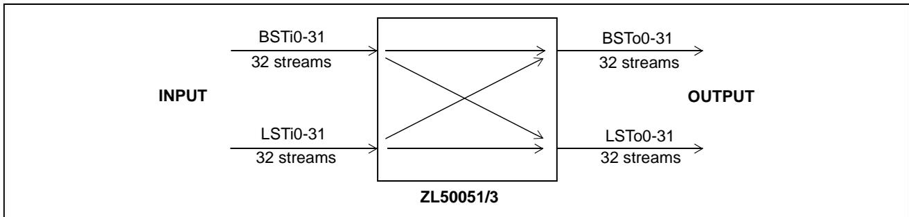
**Figure 4 - 8,192 x 8,192 Channels (8 Mbps), Unidirectional Switching**
