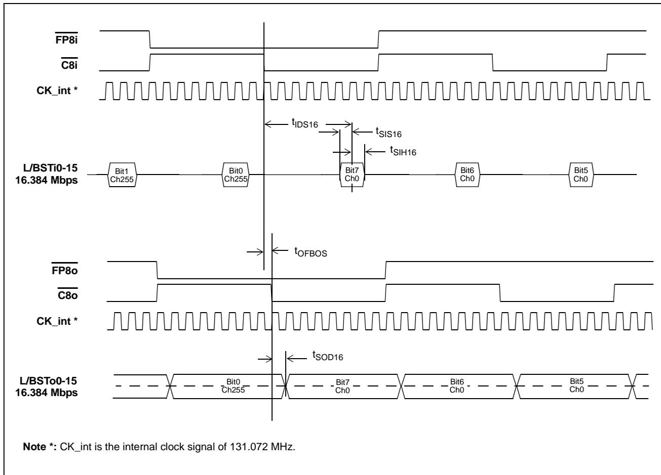
Figure 21 - ST-BUS Local/Backplane Data Timing Diagram (16 Mbps)
