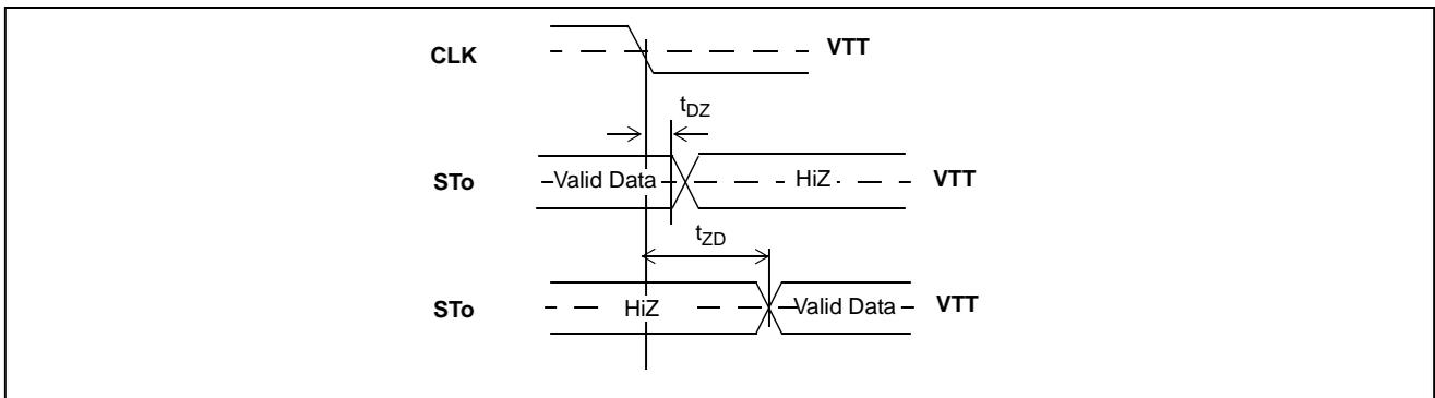
**Figure 24 - Serial Output and External Control**
