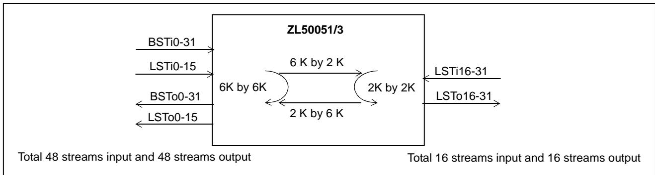
**Figure 6 - 6,144 x 2,048 Channels (8 Mbps) Blocking Bi-directional Configuration**
