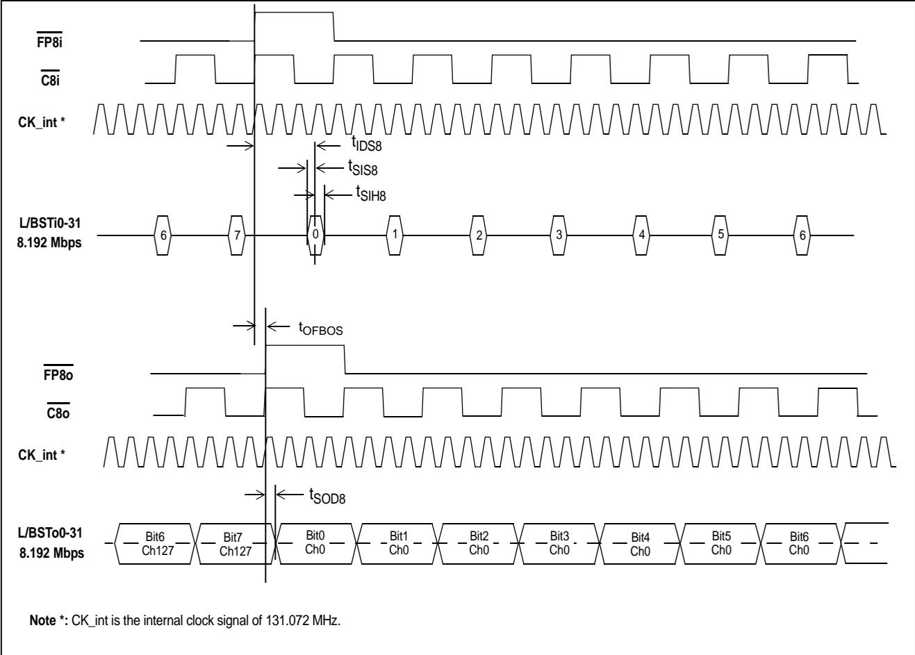
Figure 22 - GCI-Bus Local/Backplane Data Timing Diagram (8 Mbps)
