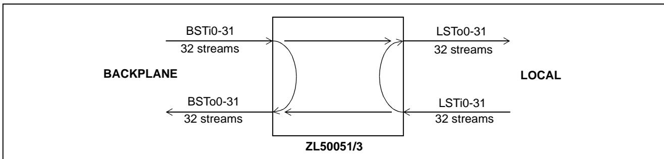
**Figure 5 - 4,096 x 4,096 Channels (8 Mbps), Bi-directional Switching**
