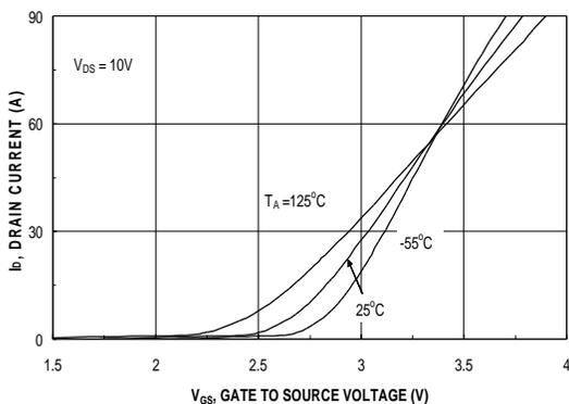
Figure 5. Transfer Characteristics
