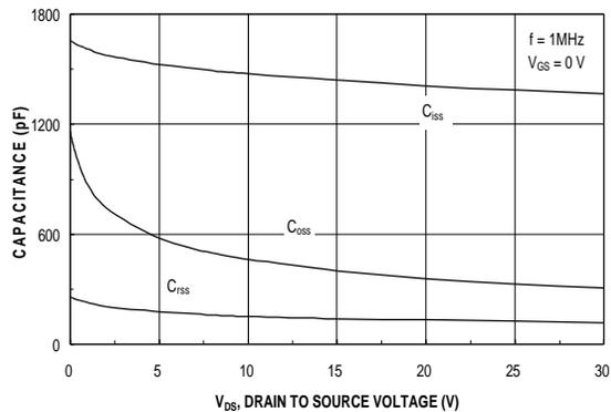
Figure 8. Capacitance Characteristics
