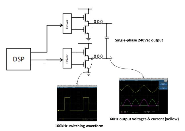
Figure 6. Typical Waveforms
