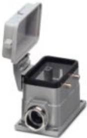
Box mounting base, with single locking latch, height 52 mm, with screw connection, 1x Pg16, with protective covers
