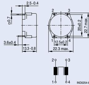
Tolerances to ISO 2768-C unless otherwise noted. Dimensions in mm.
