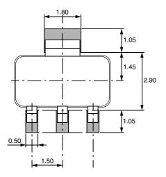
Fig. 4-2: Recommended footprint SOT89B-3, Dimensions in mm
