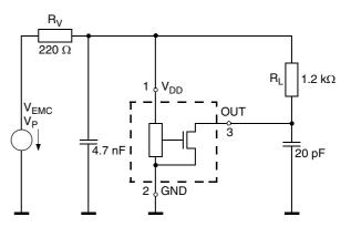
Fig. 5–1: Test circuit for EMC investigation
