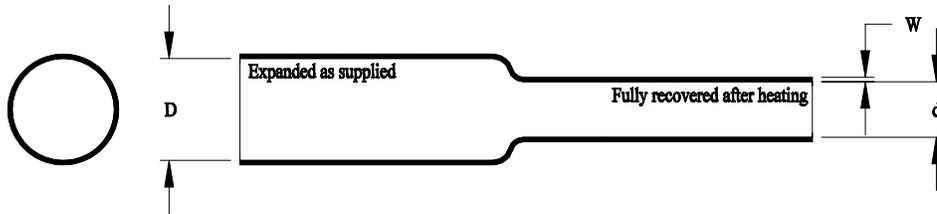
This specification covers the requirements for one type of single wall, electrical insulating, extruded tubing whose diameter will reduce to a predetermined size upon application of heat in excess of 121° C (250° F).
