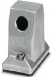
HEAVYCON ADVANCE sleeve housing, B6, with stainless steel screw locking (Allen screw), salt-water-resistant aluminum, height 93.7 mm, with 1x M32 thread, lateral cable outlet, without surface, conductive seal (EMC properties)
