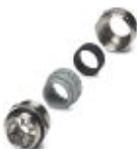
EMC screw connection up to 5 bar, thread length: 9 mm, cable diameter: 11.0 - 21.0 mm, WAF 36, screw connection: M32
