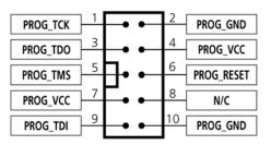
Figure 4.9.1 - Atmel 10-way IDC Header (J8) viewed from above
