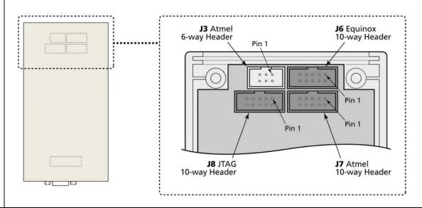
b Connect the ISP cable to the ISP Header on your Target System
