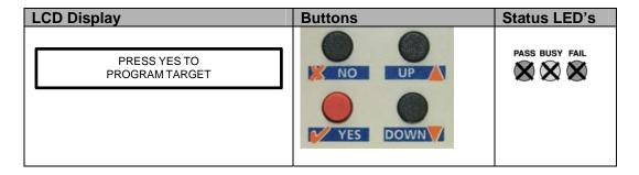
This mode is ideal for both field and production ISP requirements as the programming data is held locally in FLASH memory on the programmer so a PC is not required.
