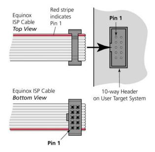
Pin 1 of the ISP cable can be determined by looking for a small arrow on the plastic part of the ISP female plug. If the cable has a RED stripe on one cable, this usually also indicates pin 1.
