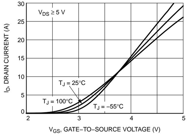
Figure 2. Transfer Characteristics
