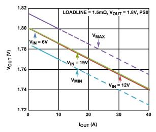
FIGURE 2. LOAD LINE REGULATION
