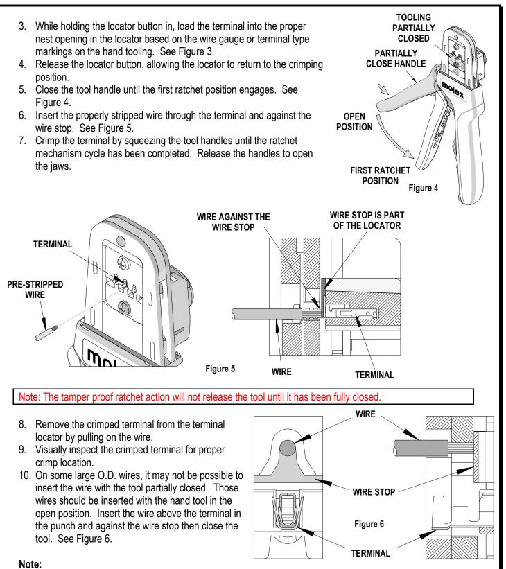
A crimp height chart is provided with this manual as <u>Reference Only.</u> Due to the wide range of wires, strands, insulation diameters, and durometers available, actual crimp height measurements may very slightly. An occasional, destructive, pull force test should be performed to check hand tool crimp. Pull Force value <u>Must</u> exceed the Minimum pull force specifications listed.
