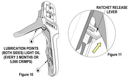
machine oil. Do not oil excessively. The tool was engineered for durability but like any other equipment it needs cleaning and lubrication for a maximum service life of trouble free crimping. Light oil (such as 30 weight automotive oil) used at the oil points, every 5,000 crimps or 3 months, will significantly enhance the tool life.
