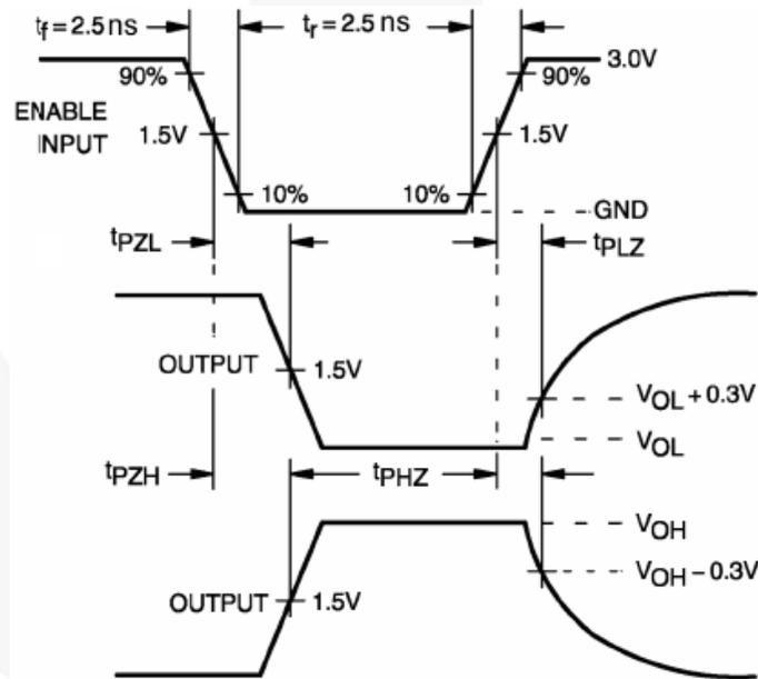
**Figure 4. AC Waveforms**
