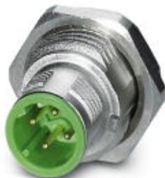
Bus system flush-type plug, with green contact carrier, 4-pos., M12 SPEEDCON, shielded, D-coded, rear/screw mounting with M16 thread, with straight solder connection
