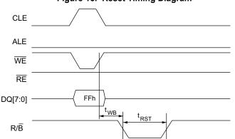
Figure 16. Reset Timing Diagram
