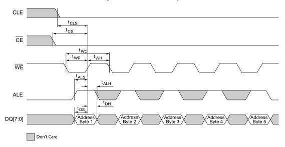
Figure 4. Address Latch Cycle
