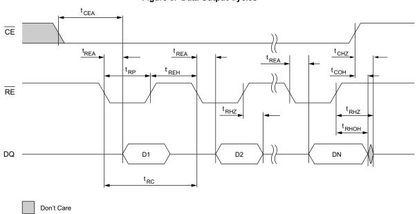
Figure 6. Data Output Cycles
