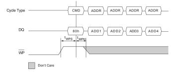
Figure 22. Write Protect Enable Timing
