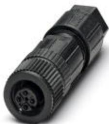
Connector, 5-position, Socket straight M12, A-coded, Push-in connection, knurl material: Plastic, external cable diameter 4 mm ... 8 mm
