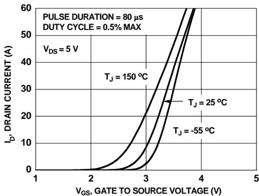
Figure 5. Transfer Characteristics
