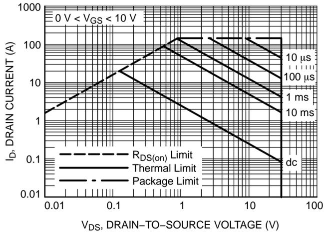
**Figure 10. Maximum Rated Forward Biased Safe Operating Area**
