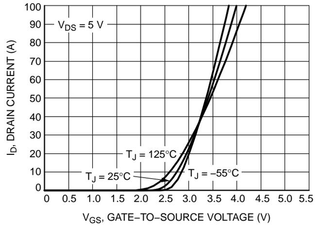
Figure 2. Transfer Characteristics
