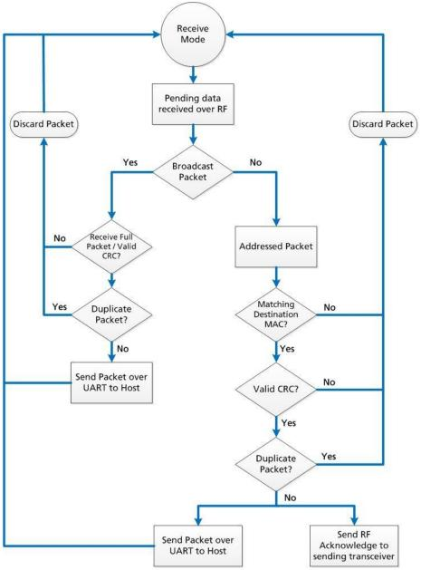
Figure 1: Pending RF Buffer Flow
