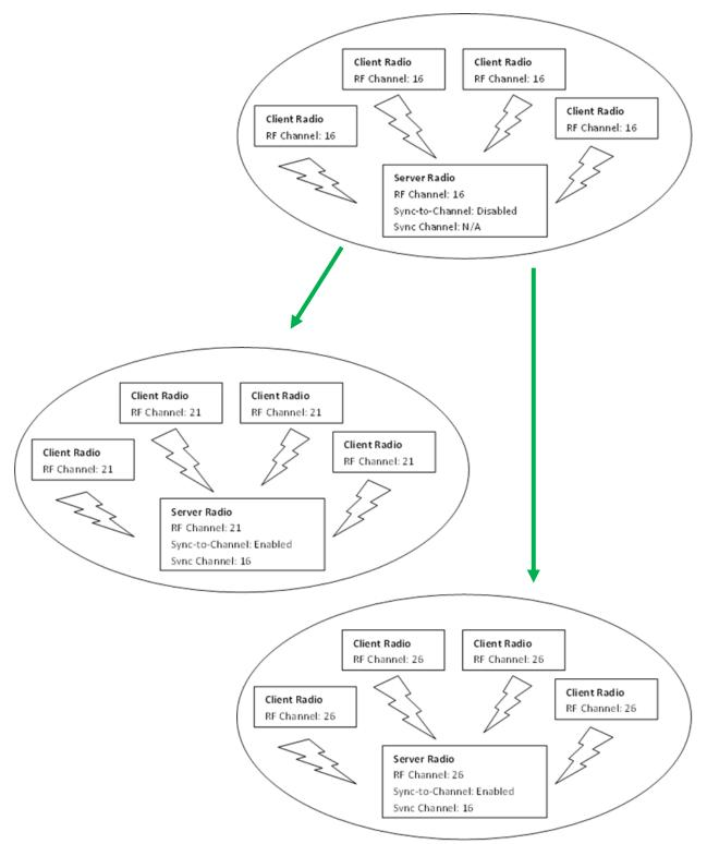
Figure 14: Sample Centralized Sync to Channel Network configuration
