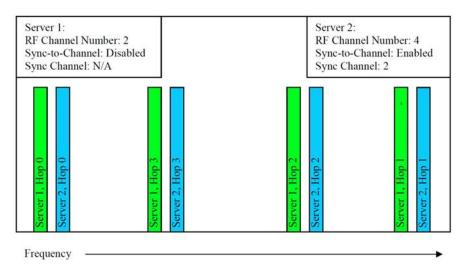
Figure 7: Two servers with Sync to Channel enabled
