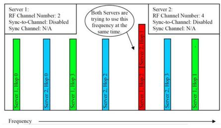
Figure 6: Two servers without Sync to Channel enabled
