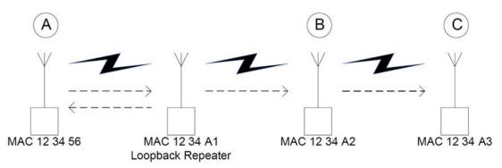
Figure 4: Loopback Repeater
