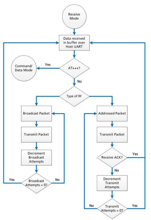
Figure 2: Pending Data in Buffer Flow
