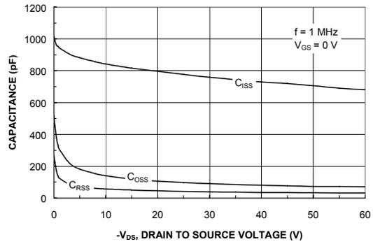
Figure 8. Capacitance Characteristics.
