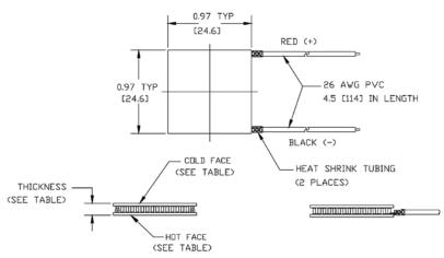
Ceramic Material: Alumina (Al<sub>2</sub>O<sub>3</sub>)
