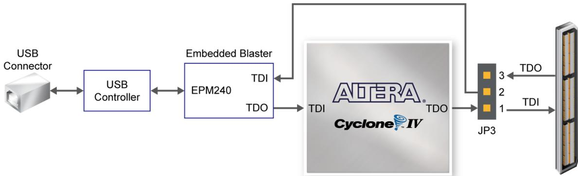
**Figure 4-1 The JTAG chain on DE2-115 board**
