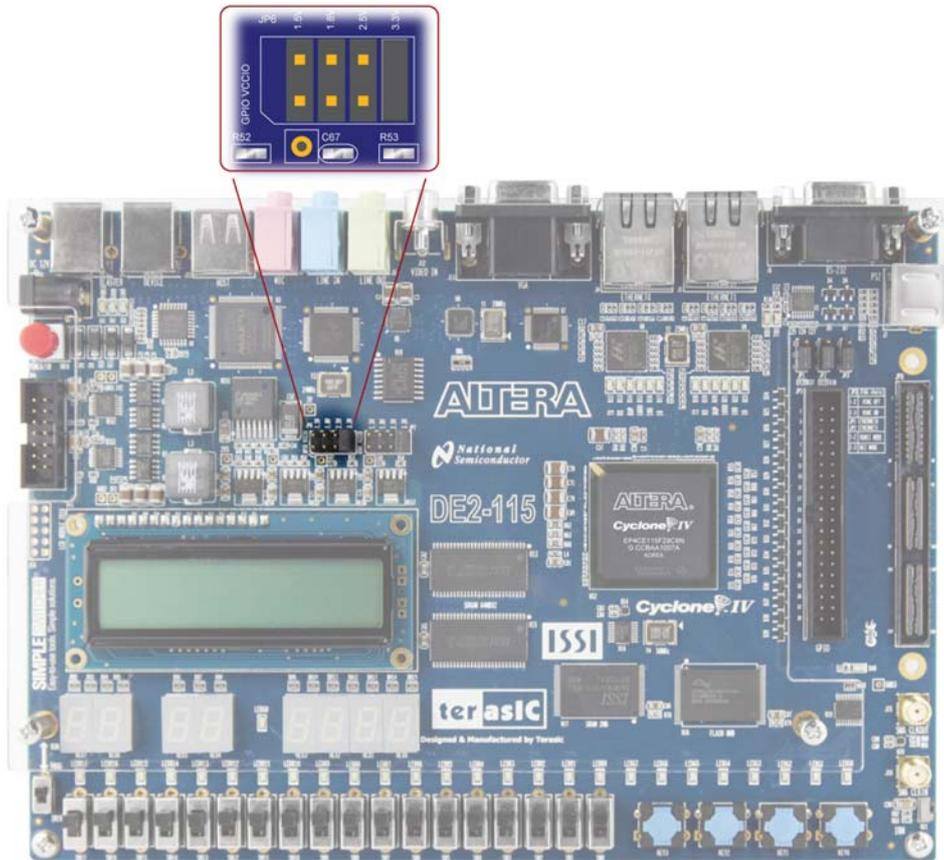
**Figure 4-17** GPIO VCCIO supply voltage setting header
