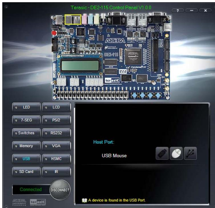
**Figure 3-8 USB Mouse Monitoring Tool**
