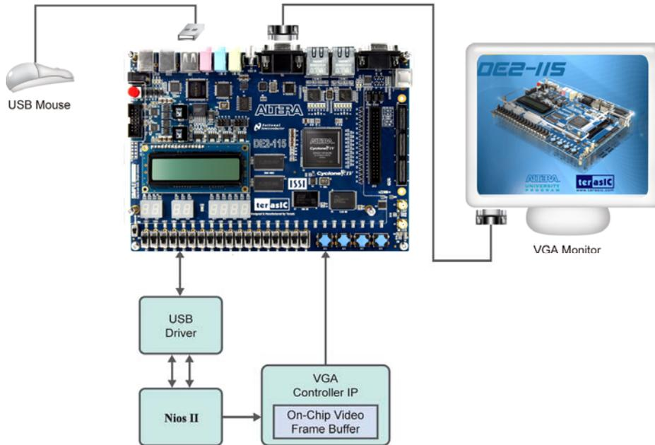
Figure 6-4 The setup for the USB paintbrush demonstration
