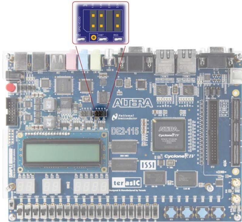
Figure 4-13 HSMC VCCIO supply voltage setting header
