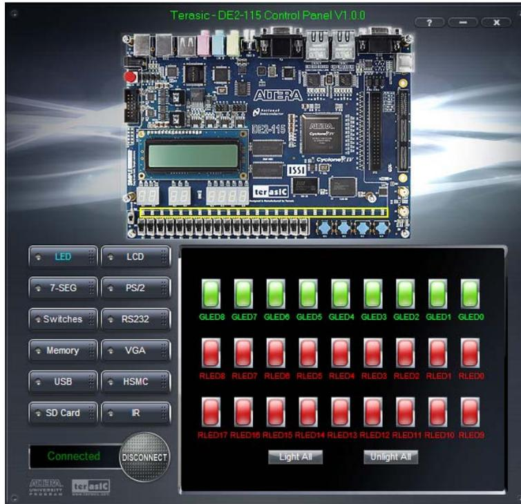
**Figure 3-3 Controlling LEDs**
