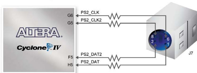
Figure 4-25 Connection between FPGA and PS/2
