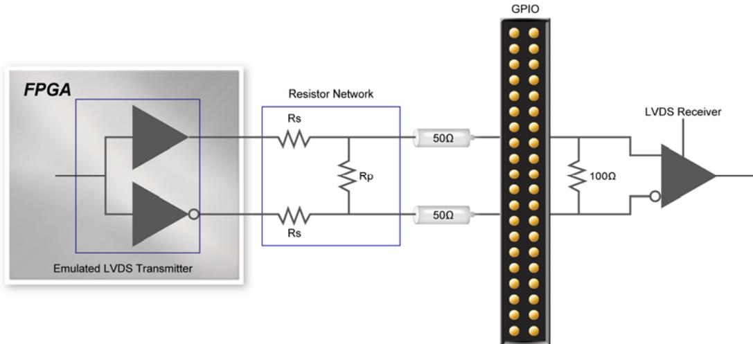
Figure 4-19 Using Emulated LVDS on GPIO
