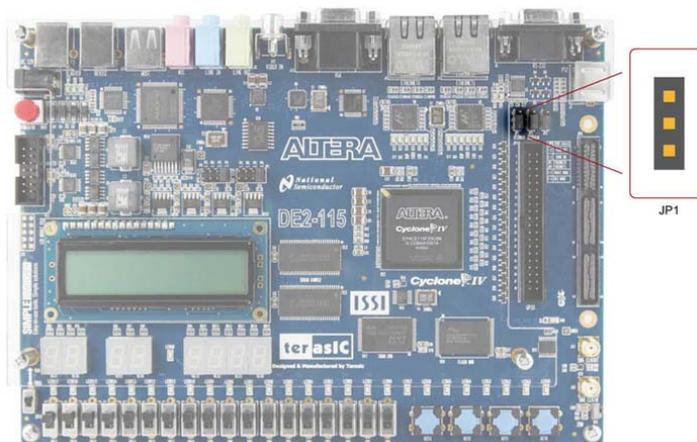
**Figure 4-28 Working mode setup header for Ethernet PHY**
