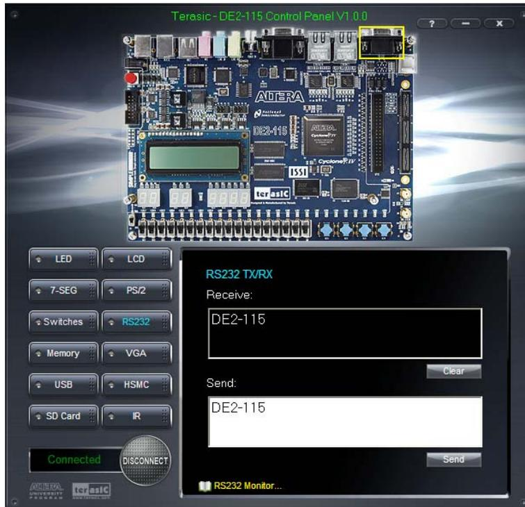
**Figure 3-11 RS-232 Serial Communication**
