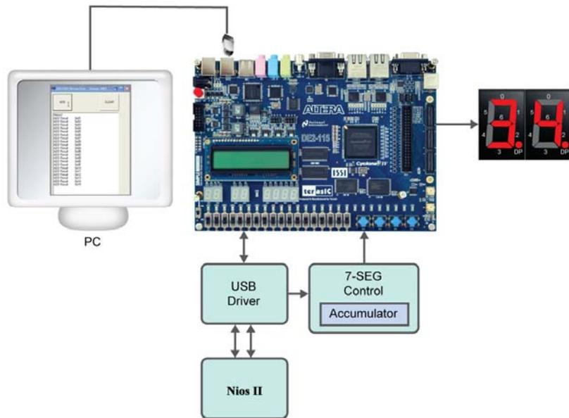
Figure 6-6 Setup for the USB device demonstration
