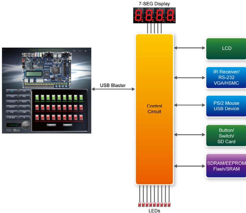
**Figure 3-2 The DE2-115 Control Panel concept**
