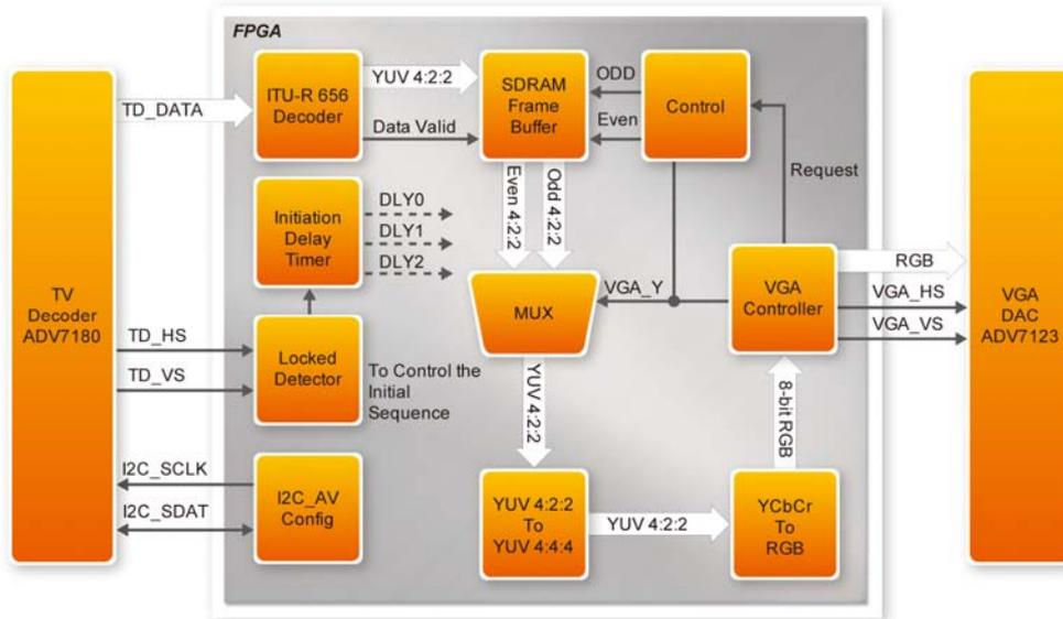
Figure 6-1 Block diagram of the TV box demonstration
