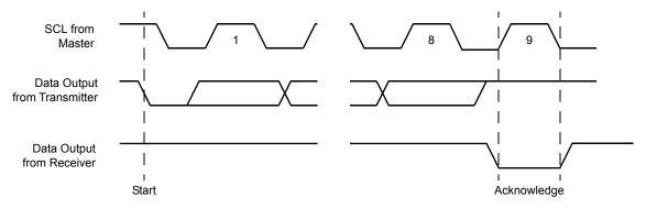
Figure 9. Byte Write Sequence
