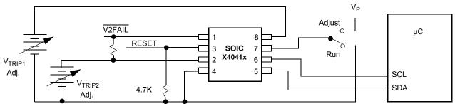
Figure 5. V<sub>TRIPX</sub> Set/Reset Sequence (X = 1, 2)
