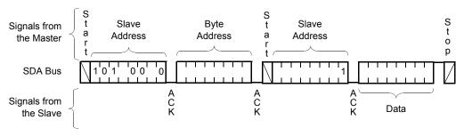
One bit of the slave command byte is a R/W bit. The R/W bit of the Slave Address Byte defines the operation to be performed. When the R/W bit is a one, then a read operation is selected. A zero selects a write operation.
