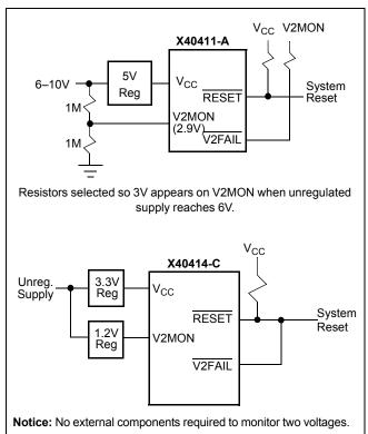
Figure 2. V<sub>TRIPX</sub> Set/Reset Conditions
