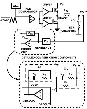
FIGURE 7. VOLTAGE-MODE BUCK CONVERTER COMPENSATION DESIGN
