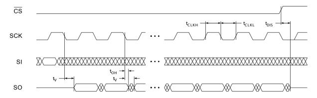
Figure 14-3. WP Timing for Write Status Register Byte 1 Command When SPRL = 1
