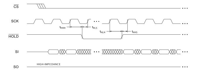
Figure 14-5. HOLD Timing – Serial Output
