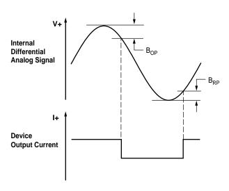
Figure 6: Peak Detecting Switchpoint Detail
