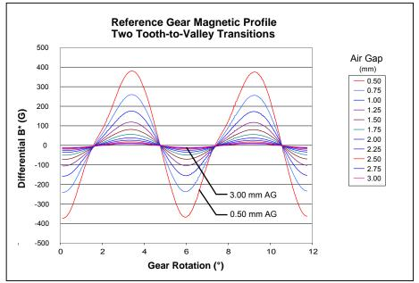
\*Differential B corresponds to the calculated difference in the magnetic field as sensed simultaneously at the two Hall elements in the device ( $B_{DIFF} = B_{E1} - B_{E2}$ ).
