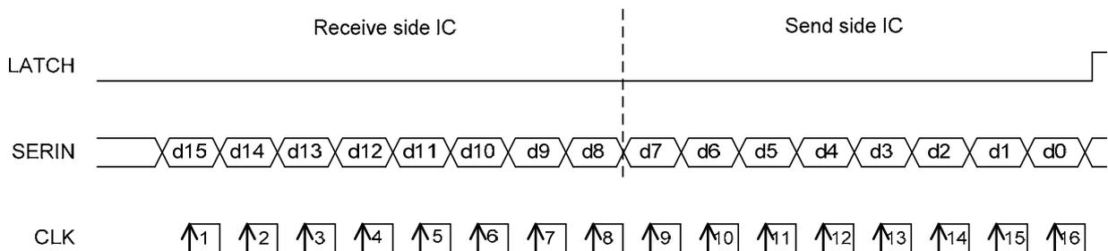
Figure 17. Cascade Connection
