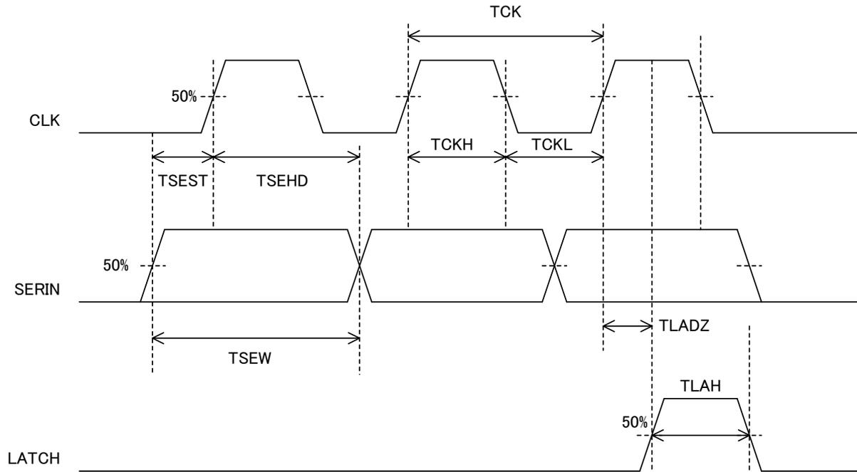
Figure 18. Timing Chart of Input Signal
