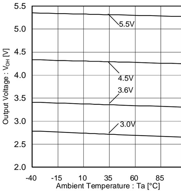
Figure 10. SEROUT High Side Voltage (Temperature characteristic @  $I_{SO}=-4mA$ )
