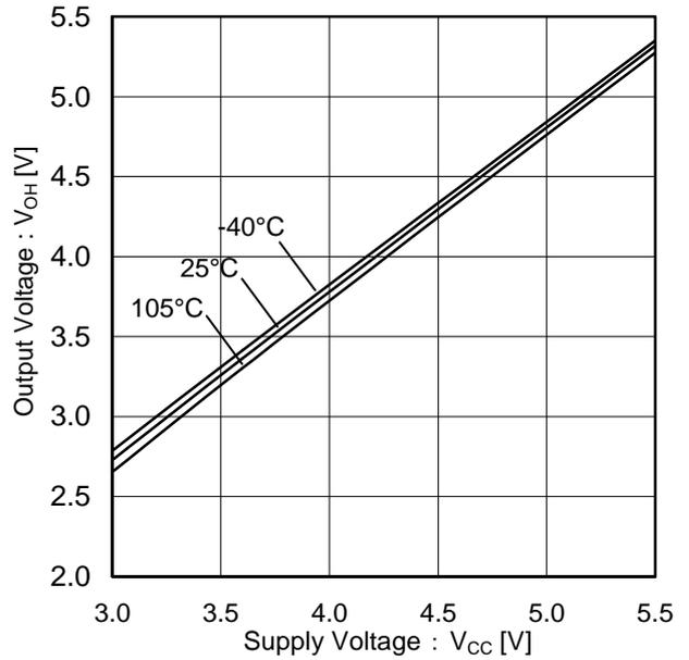
Figure 9. SEROUT High Side Voltage ( $V_{CC}$  characteristic @  $I_{SO}=-4mA$ )
