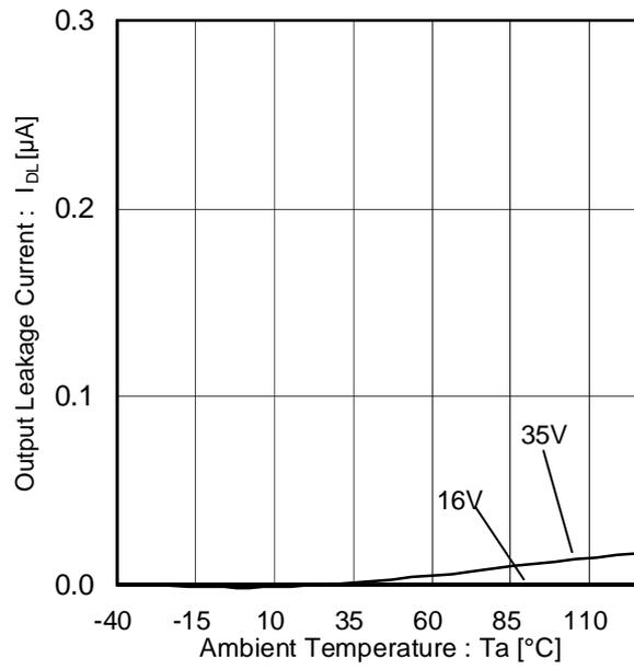
Figure 13. Output Leakage Current (Temperature characteristic)
