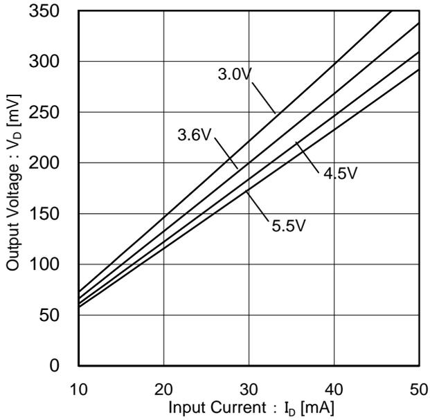
Figure 8. Output ON Resistance ( $I_b$  characteristic)
