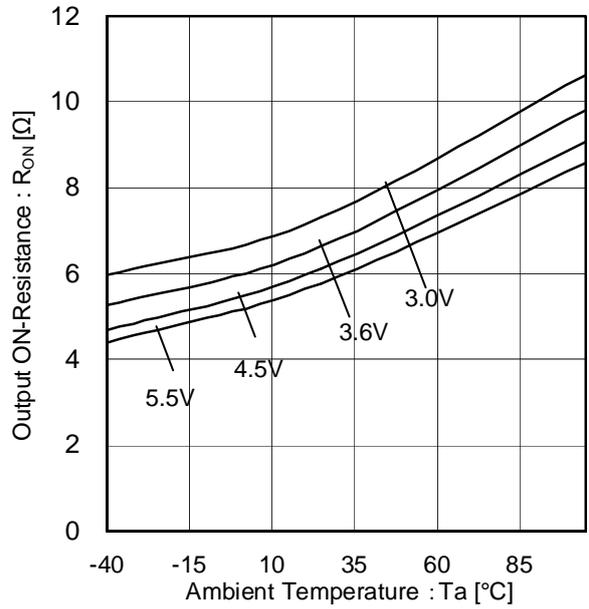
Figure 7. Output ON Resistance (Temperature characteristic @ ID=20mA)
