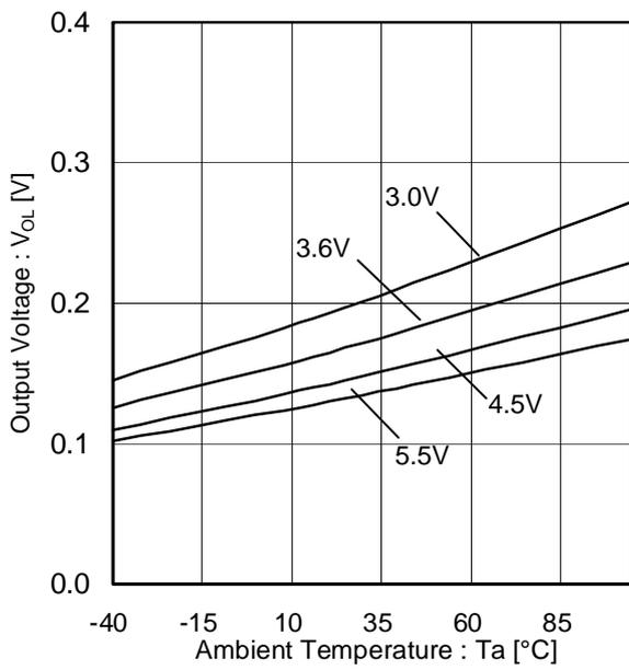
Figure 12. SEROUT Low Side Voltage (Temperature characteristic @ ISO=4mA)
