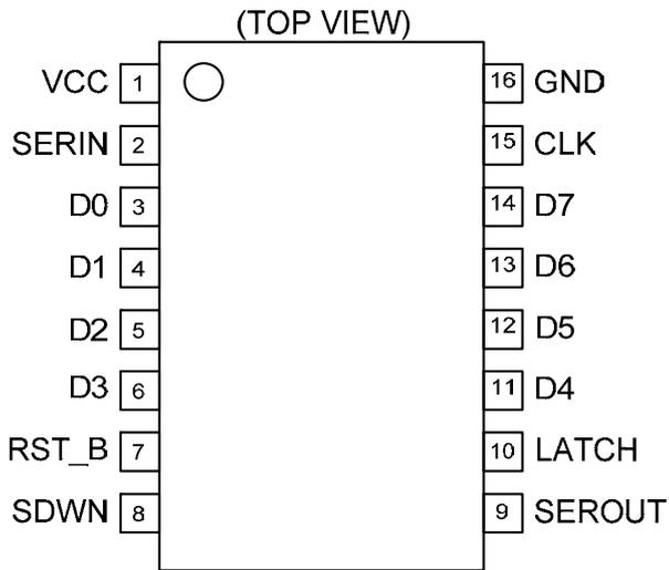
Figure 2. Pin Configuration
