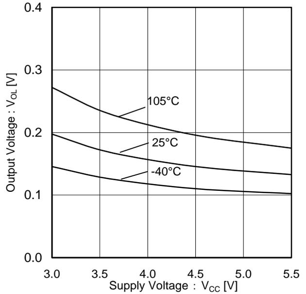
Figure 11. SEROUT Low Side Voltage ( $V_{CC}$  characteristic @  $I_{SO}=4mA$ )
