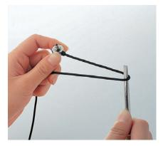
A cabtyre cable is used, so that the sensor cable will not break like fibers.
