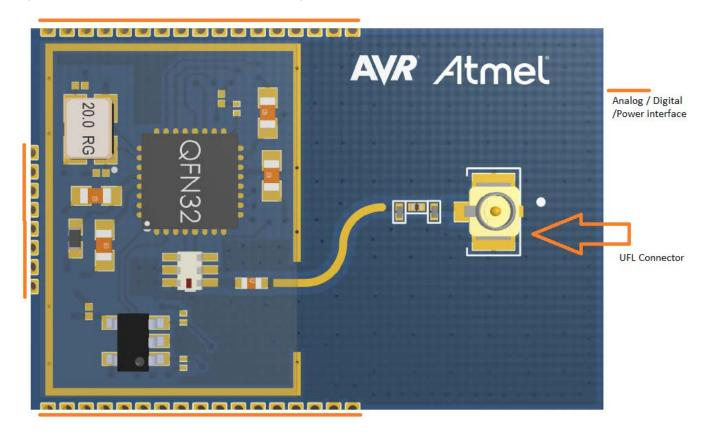
This ZigBit module contains Atmel's AT86RF212B 900MHz ISM band Transceiver for ZigBee and IEEE 802.15.4 [1].
