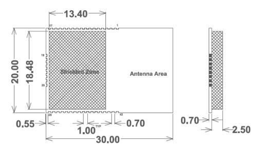
Atmel ATZB-RF212B -Pinout
