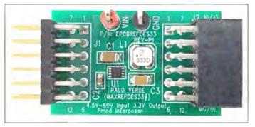
solution can be used in many different types of power applications, such as 4–20mA current loops, HVAC and building control, high-voltage LDO replacement, general-purpose point-of-load, etc. In this reference design, the MAX15062 performs in 24V input applications, such as industrial sensors, process control, etc.
