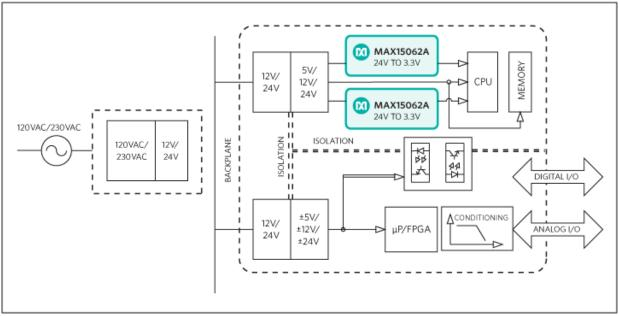
Figure 1. Typical industrial control power system diagram.
