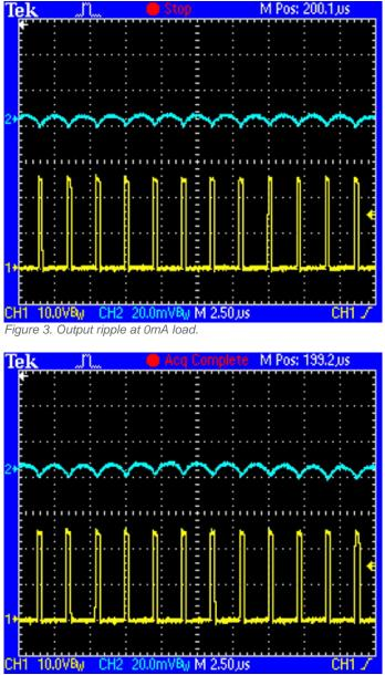
Figure 4. Output ripple at 300mA load.
