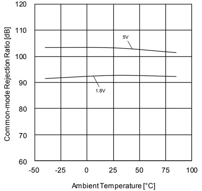
Figure 18. Common-mode Rejection Ratio vs Ambient Temperature
