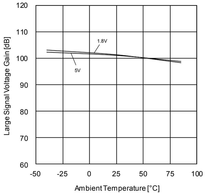
Figure 44. Large Signal Voltage Gain vs Ambient Temperature (R<sub>L</sub>=2kΩ)
