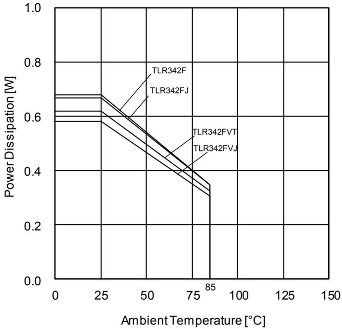
Figure 29. Power Dissipation vs Ambient Temperature (Derating Curve)
