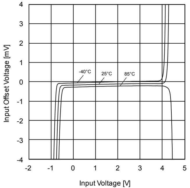
Figure 42. Input Offset Voltage vs Input Voltage (V<sub>DD</sub>=5V)
