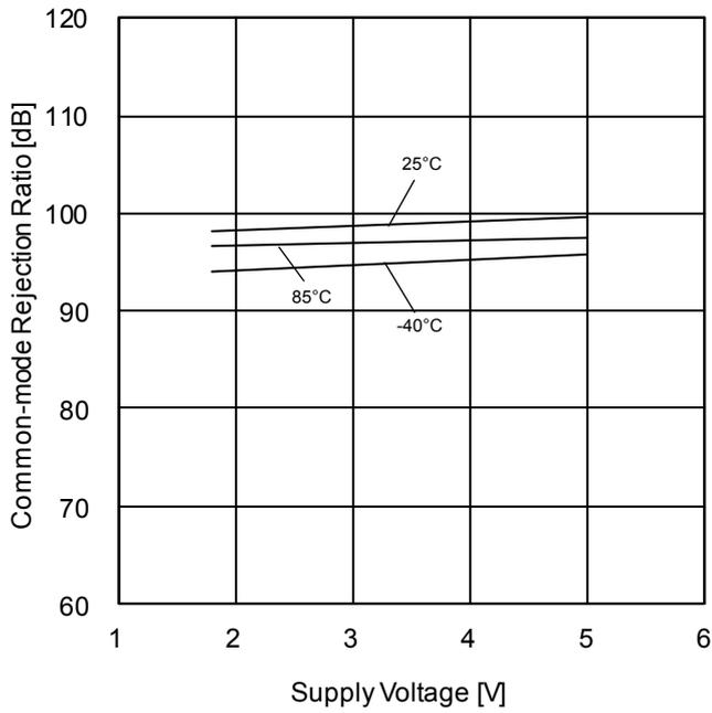
Figure 45. Common-mode Rejection Ratio vs Supply Voltage ( $V_{DD}=1.8V$ )
