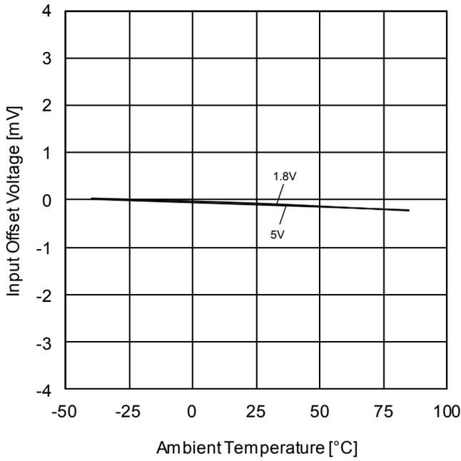
Figure 41. Input Offset Voltage vs Ambient Temperature
