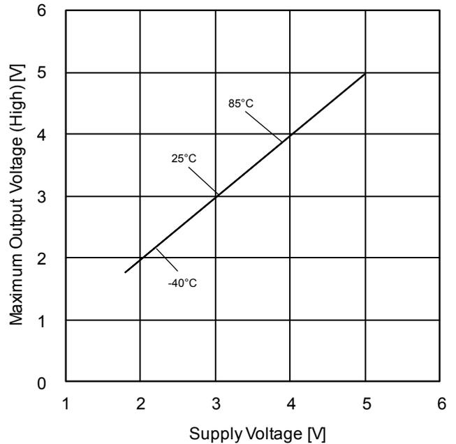
Figure 4. Maximum Output Voltage High vs Supply Voltage (RL=2kΩ)
