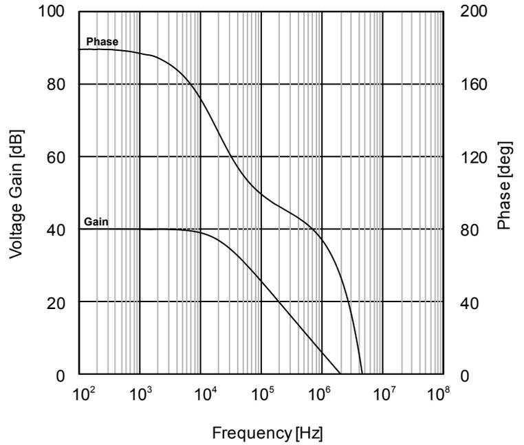
Figure 22. Voltage Gain, Phase vs Frequency (V<sub>DD</sub>=1.8V, T<sub>A</sub>=25°C)
