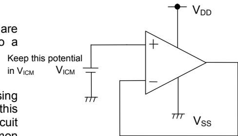
Figure 78. Example of Application Circuit for Unused Op-amp
