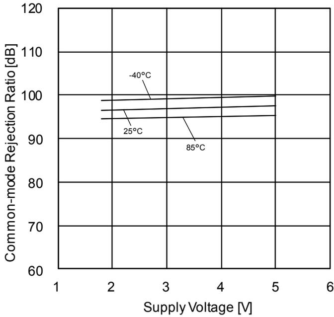
Figure 67. Common-mode Rejection Ratio vs Supply Voltage
