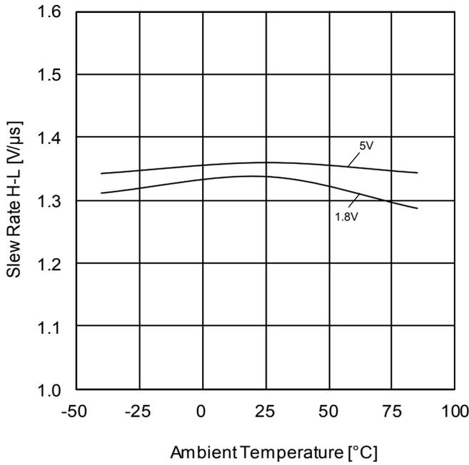
Figure 21. Slew Rate H-L vs Ambient Temperature
