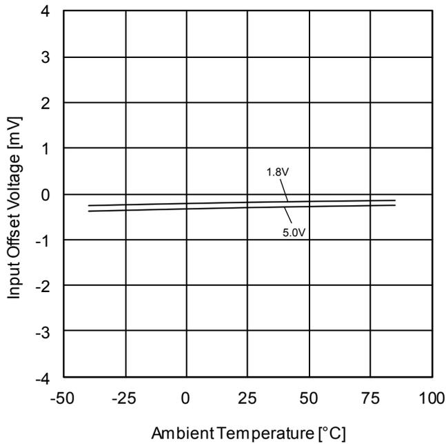
Figure 63. Input Offset Voltage vs Ambient Temperature
