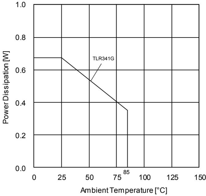
Figure 1. Power Dissipation vs Ambient Temperature (Derating Curve)
