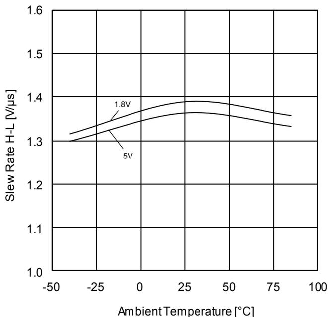
Figure 71. Slew Rate H-L vs Ambient Temperature
