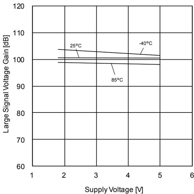
Figure 65. Large Signal Voltage Gain vs Supply Voltage (R<sub>L</sub>=2kΩ)
