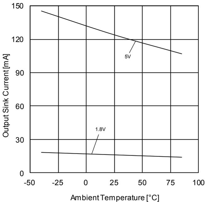
Figure 61. Output Sink Current vs Ambient Temperature ( $V_{OUT}=V_{DD}$ )
