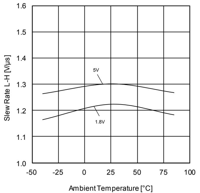
Figure 20. Slew Rate L-H vs Ambient Temperature
