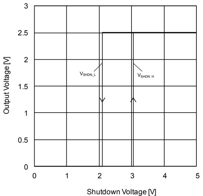
Figure 28. Output Voltage vs Shutdown Voltage
