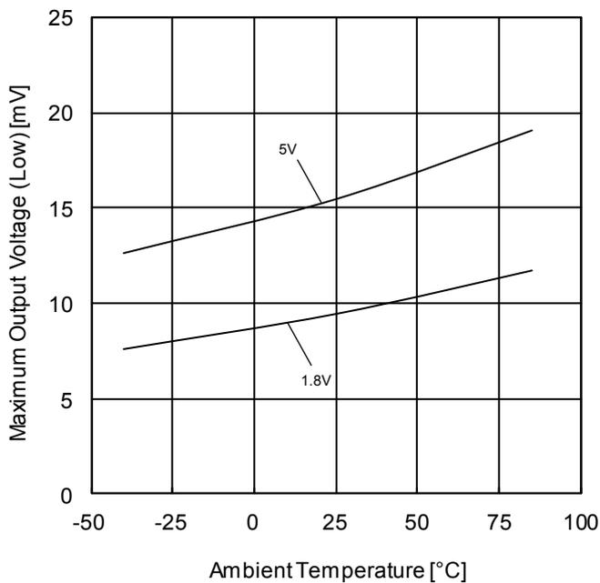
Figure 57. Maximum Output Voltage (Low) vs Ambient Temperature ( $R_L=2k\Omega$ )
