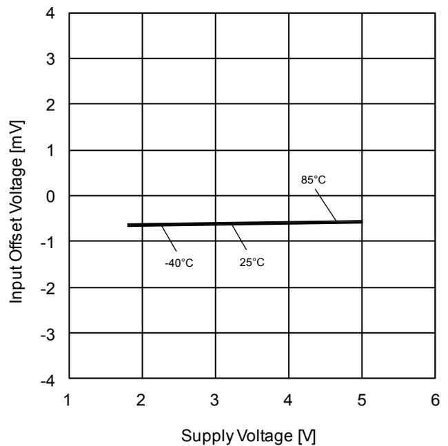
Figure 12. Input Offset Voltage vs Supply Voltage
