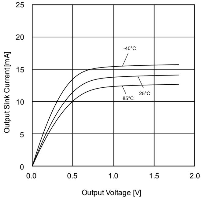
Figure 10. Output Sink Current vs Output Voltage ( $V_{DD}=1.8V$ )
