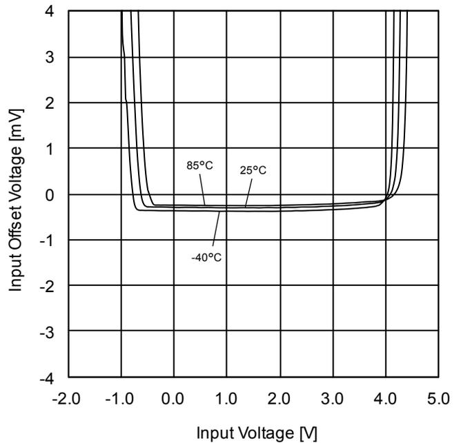
Figure 64. Input Offset Voltage vs Input Voltage (V<sub>DD</sub>=5V)
