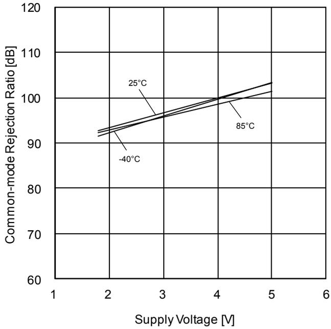
Figure 17. Common-mode Rejection Ratio vs Supply Voltage ( $V_{DD}=1.8V$ )
