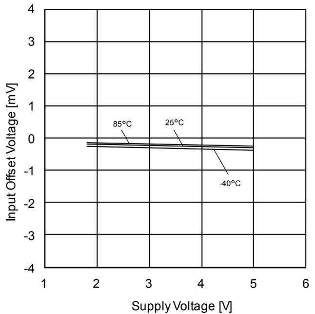
Figure 62. Input Offset Voltage vs Supply Voltage
