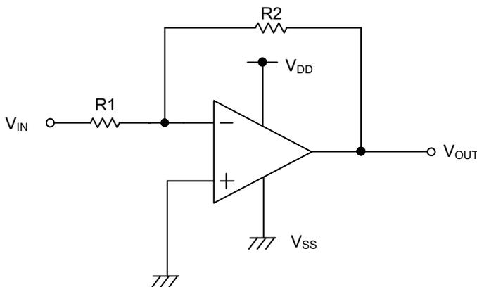
Figure 80. Inverting Amplifier Circuit
