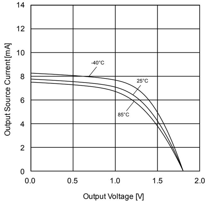
Figure 36. Output Source Current vs Output Voltage ( $V_{DD}=1.8V$ )
