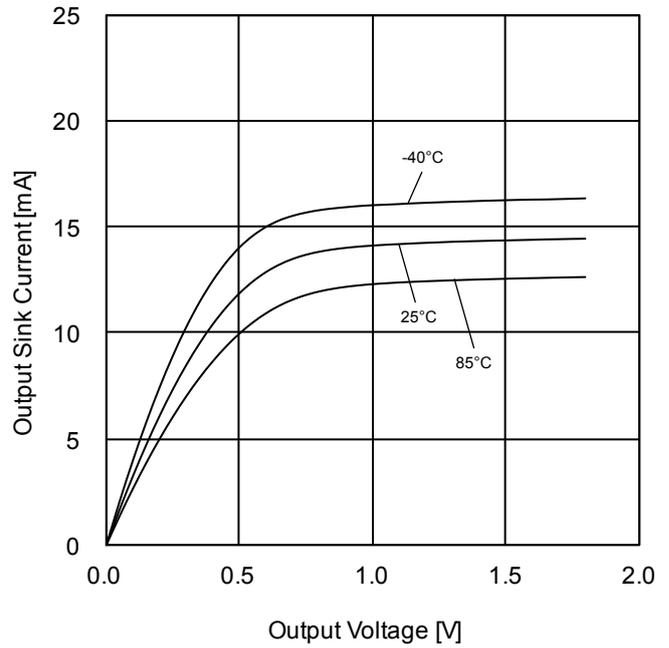
Figure 38. Output Sink Current vs Output Voltage ( $V_{DD}=1.8V$ )
