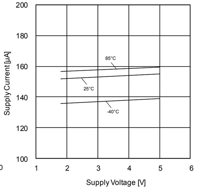
Figure 30. Supply Current vs Supply Voltage
