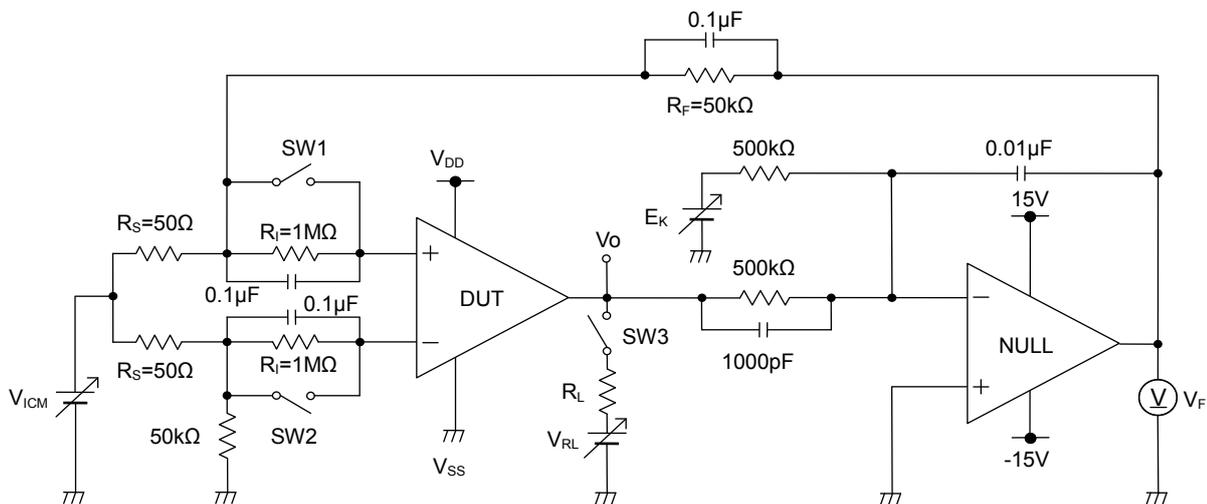
Figure 73. Test Circuit 1
