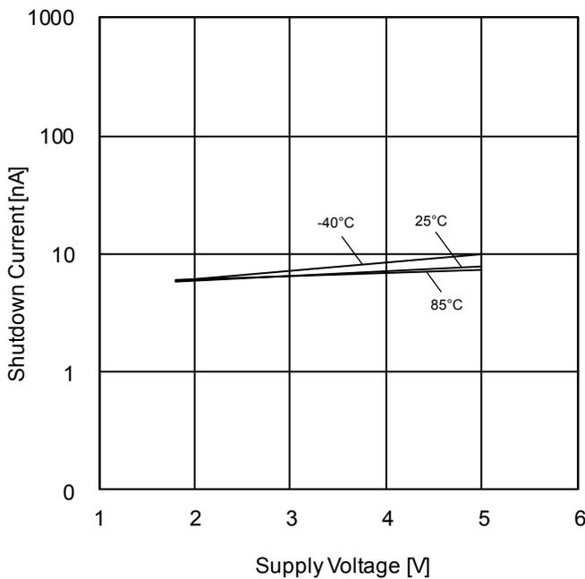
Figure 23. Shutdown Current vs Supply Voltage (V<sub>SHDN</sub>=0V)
