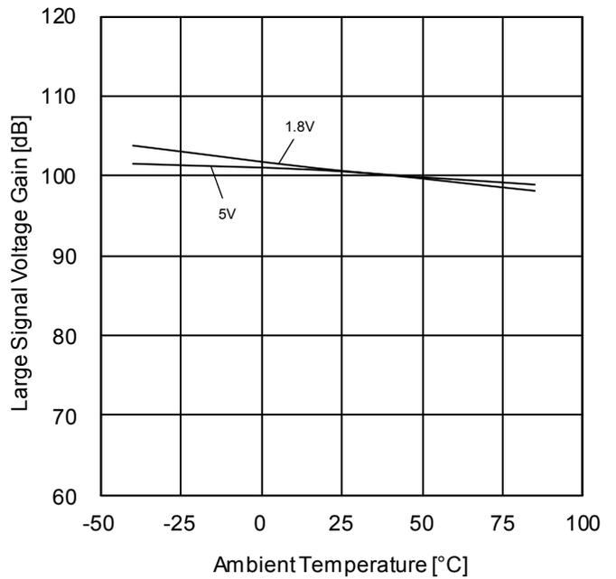
Figure 66. Large Signal Voltage Gain vs Ambient Temperature (R<sub>L</sub>=2kΩ)
