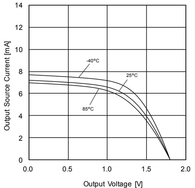
Figure 58. Output Source Current vs Output Voltage ( $V_{DD}=1.8V$ )
