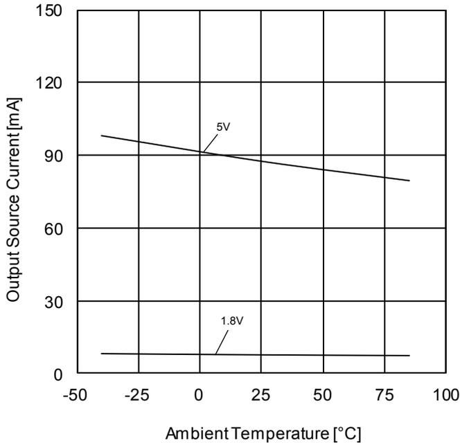
Figure 9. Output Source Current vs Ambient Temperature ( $V_{OUT}=0V$ )
