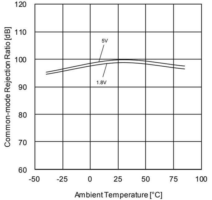
Figure 68. Common-mode Rejection Ratio vs Ambient Temperature
