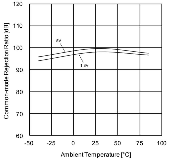
Figure 46. Common-mode Rejection Ratio vs Ambient Temperature
