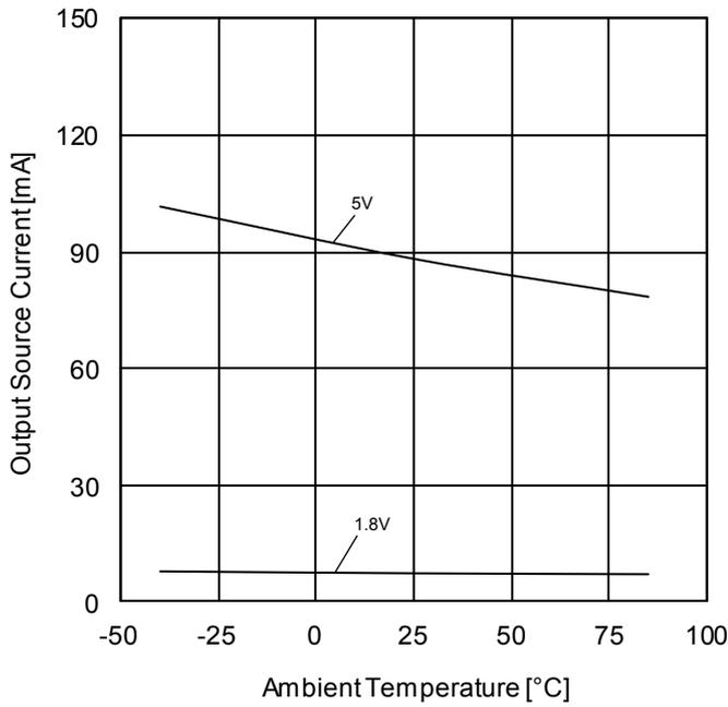
Figure 59. Output Source Current vs Ambient Temperature ( $V_{OUT}=0V$ )
