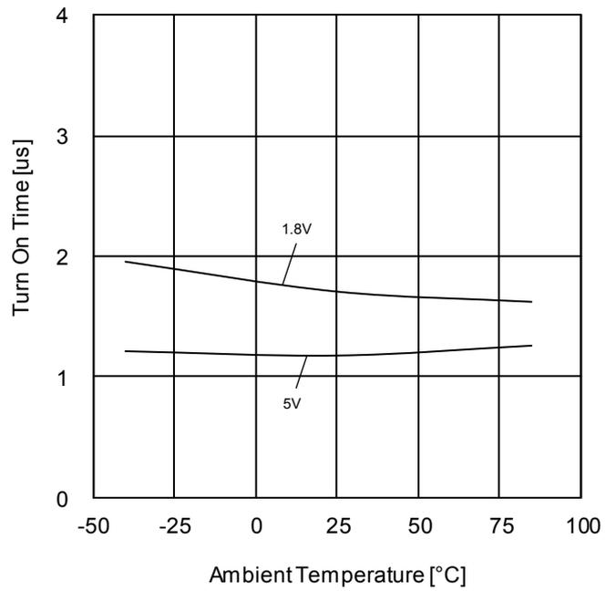
Figure 26. Turn On Time vs Ambient Temperature
