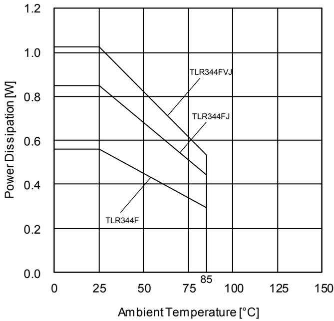
Figure 51. Power Dissipation vs Ambient Temperature (Derating Curve)
