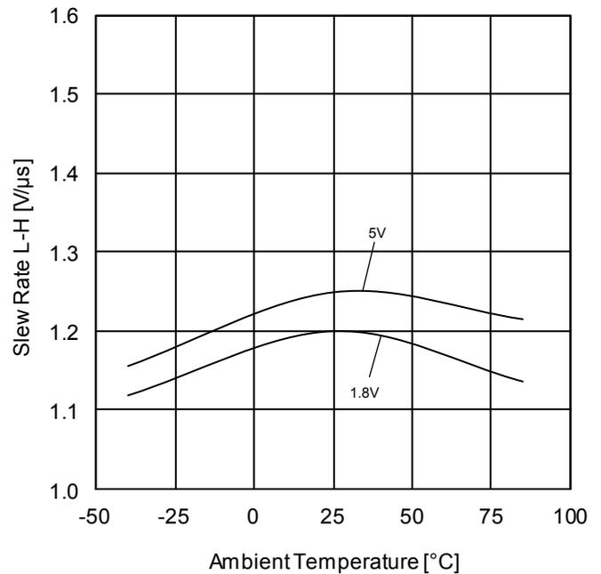
Figure 70. Slew Rate L-H vs Ambient Temperature
