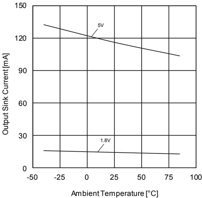
Figure 11. Output Sink Current vs Ambient Temperature ( $V_{OUT}=V_{DD}$ )
