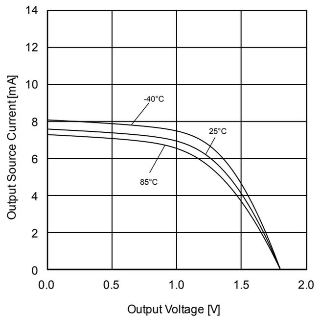
Figure 8. Output Source Current vs Output Voltage ( $V_{DD}=1.8V$ )
