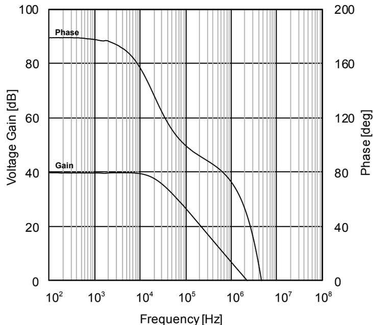
Figure 72. Voltage Gain, Phase vs Frequency (V<sub>DD</sub>=1.8V, T<sub>A</sub>=25°C)
