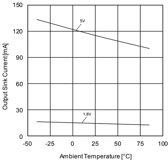
Figure 39. Output Sink Current vs Ambient Temperature ( $V_{OUT}=V_{DD}$ )
