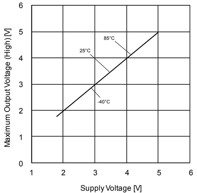
Figure 32. Maximum Output Voltage High vs Supply Voltage (R<sub>L</sub>=2kΩ)
