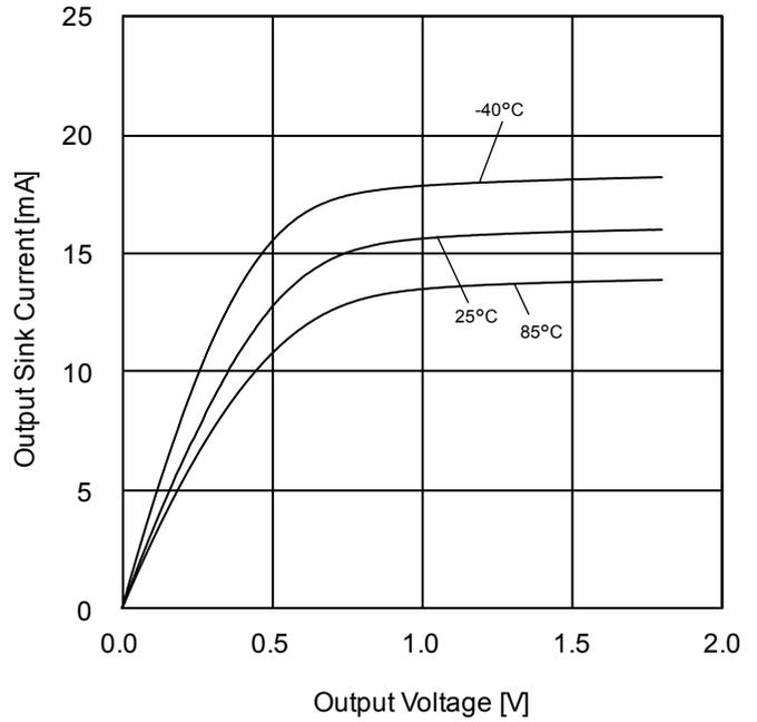
Figure 60. Output Sink Current vs Output Voltage ( $V_{DD}=1.8V$ )
