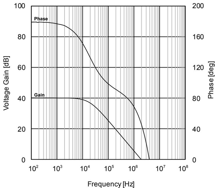
Figure 50. Voltage Gain, Phase vs Frequency (V<sub>DD</sub>=1.8V, T<sub>A</sub>=25°C)
