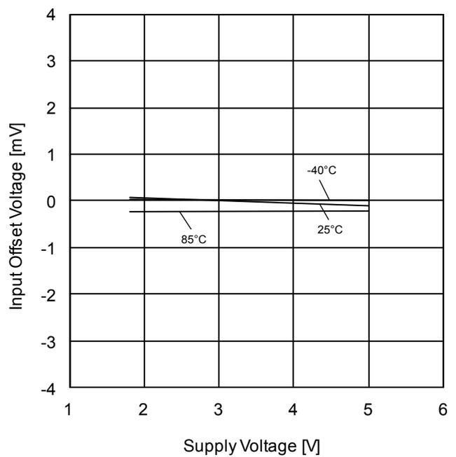
Figure 40. Input Offset Voltage vs Supply Voltage
