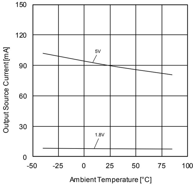
Figure 37. Output Source Current vs Ambient Temperature ( $V_{OUT}=0V$ )
