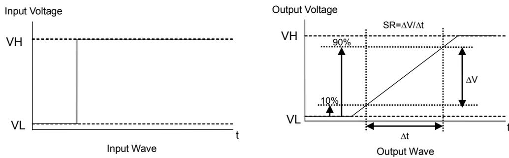
Figure 75. Slew Rate Input and Output Wave
