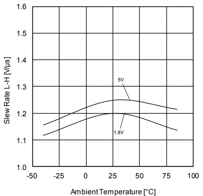
Figure 48. Slew Rate L-H vs Ambient Temperature
