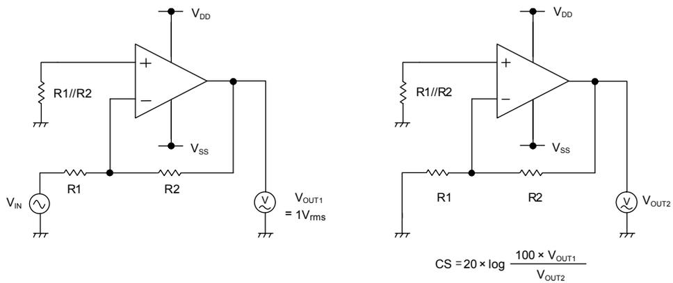
Figure 77. Test Circuit 3 (Channel Separation)
