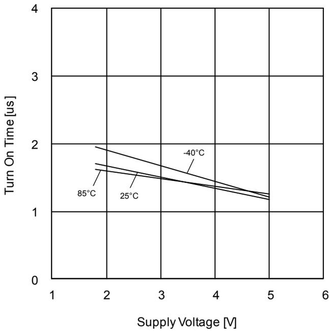
Figure 25. Turn On Time vs Supply Voltage
