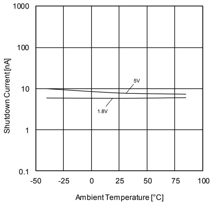
Figure 24. Shutdown Current vs Ambient Temperature (V<sub>SHDN</sub>=0V)
