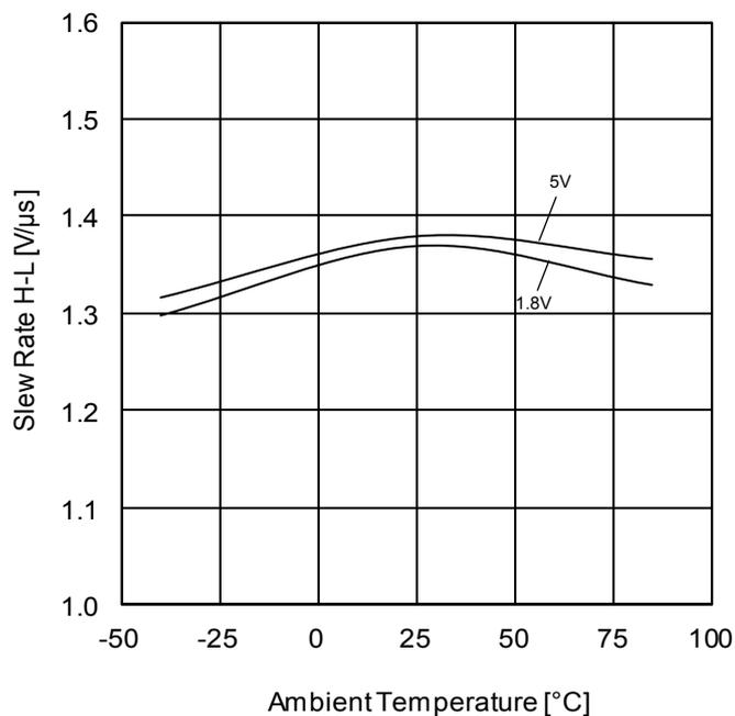
Figure 49. Slew Rate H-L vs Ambient Temperature
