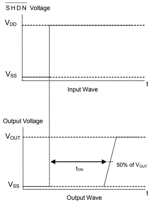
Figure 76. Turn On Time Input and Output Wave
