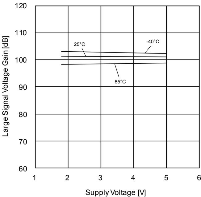
Figure 43. Large Signal Voltage Gain vs Supply Voltage (R<sub>L</sub>=2kΩ)
