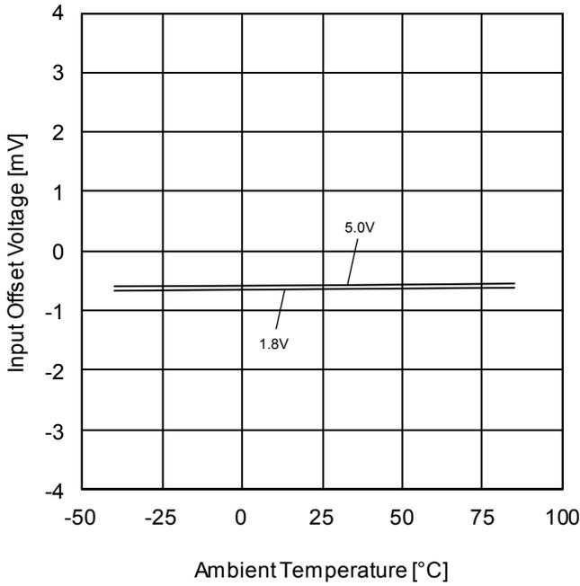
Figure 13. Input Offset Voltage vs Ambient Temperature
