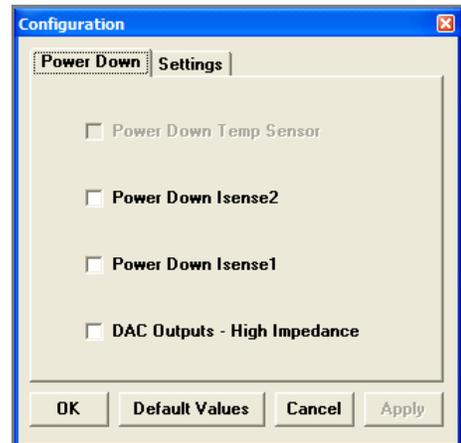
Figure 14. Power-Down Modes Available in the Configuration Window
