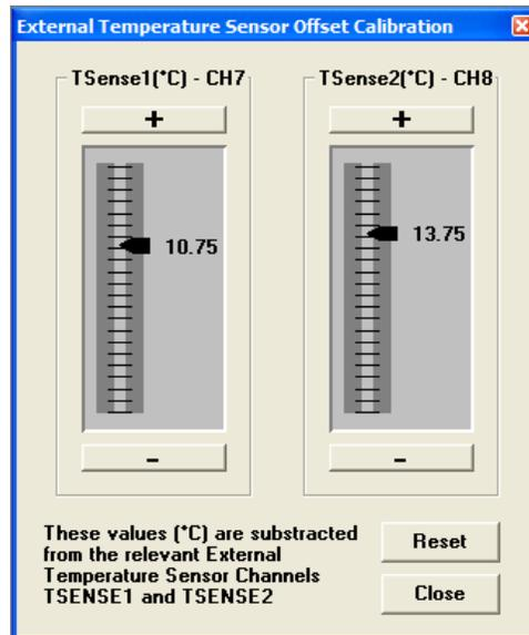
Figure 25. External Temperature Sensor Offset Calibration Window
