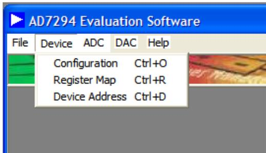
Figure 12. Device Menu of the Main Window
