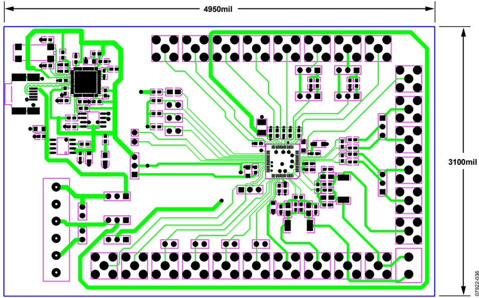
Figure 36. Evaluation Board Layout, Component Side View
