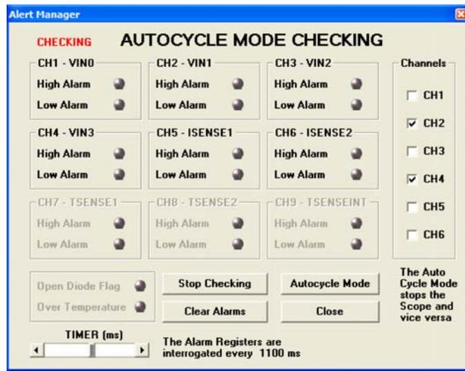
Figure 24. Autocycle Mode in the Alert Manager Window
