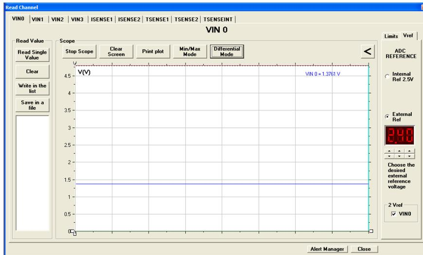
Figure 21. Vref Tab of the Read Channel Window
