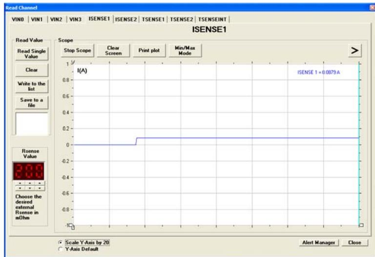
Figure 22. ISENSE1 Tab of the Read Channel Window
