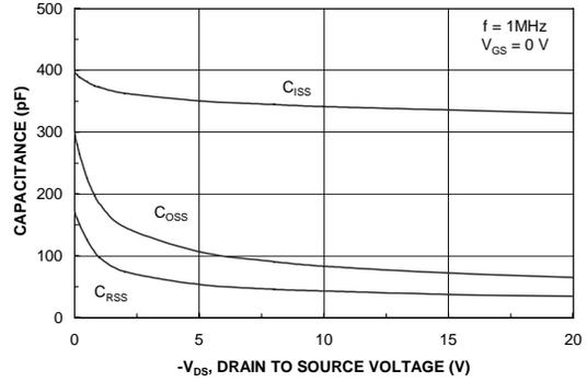
Figure 8. Capacitance Characteristics.
