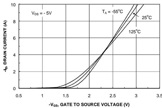
Figure 5. Transfer Characteristics.
