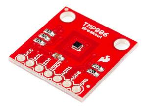
The sensor can measure temperatures between -40°C and 125°C. It can be powered with 3.3V or 5V or anything in between. It can be used with battery powered applications as it is low power and has a typical idle (quiescent) current of 240  $\mu$ A. It sports a very tiny form factor. You can interface with the chip using I<sup>2</sup>C and can have up to eight of them on the same I<sup>2</sup>C bus.
