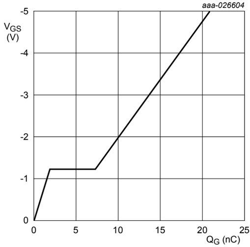
$V_{DS} = -10\text{ V}; I_D = -3\text{ A}; T_{amb} = 25\text{ }^\circ\text{C}$
