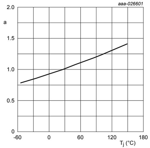
$$a = \frac{R_{DSon}}{R_{DSon(25^{\circ}C)}}$$
