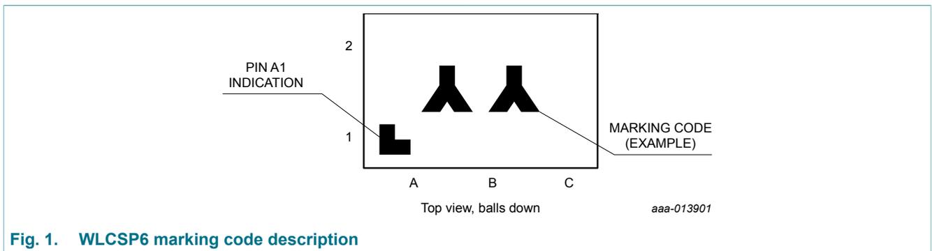
Fig. 1. WLCSP6 marking code description
