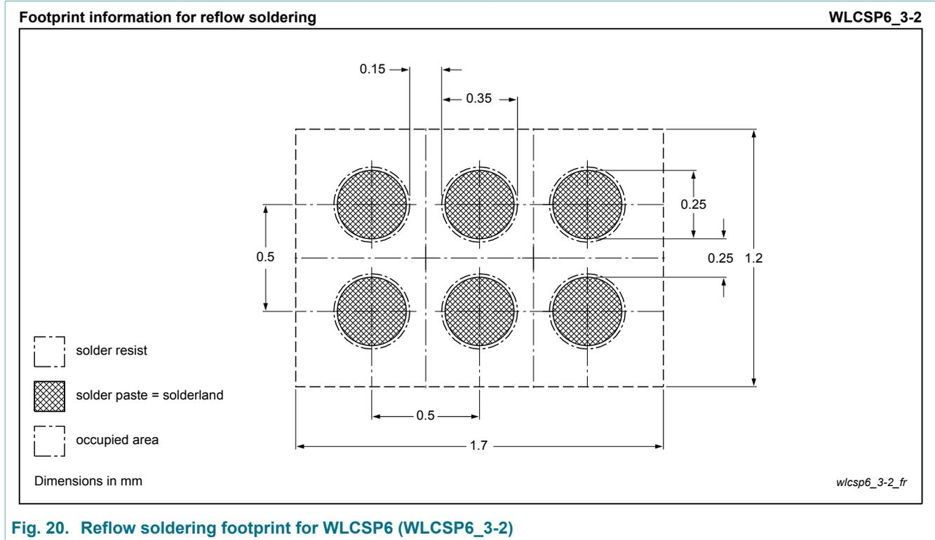
Fig. 20. Reflow soldering footprint for WLCSP6 (WLCSP6\_3-2)
