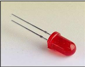
An LED is a special diode. LED stands for Light Emitting Diode. LEDs are like normal diodes, in that they only allow current to flow in one direction, however when the current is flowing the LED lights.
