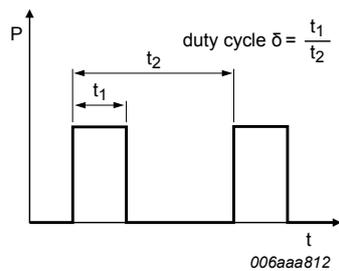
Fig. 17. Duty cycle definition
