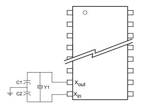
Recommended Values  $Y_1 = 32.768 \text{ kHz} (12.5 \text{ pF})$   $C_1 = 12 \text{ pF}$  $C_2 = 69 \text{ pF}$
