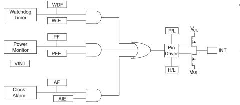
WDF - Watchdog Timer Flag WIE - Watchdog Interrupt Enable PF - Power Fail Flag PFE - Power Fail Enable AF - Alarm Flag AIE - Alarm Interrupt Enable P/L - Pulse Level H/L - High/Low
