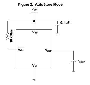
Figure 2 on page 4 shows the proper connection of the storage capacitor (V<sub>CAP</sub>) for automatic STORE operation. Refer to DC Electrical Characteristics on page 16 for the size of the V<sub>CAP</sub>. The voltage on the V<sub>CAP</sub> pin is driven to V<sub>CC</sub> by a regulator on the
