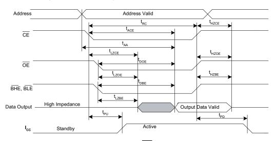
Figure 9. SRAM Read Cycle 2 (CE and OE Controlled) <sup>[30, 31, 32]</sup>
