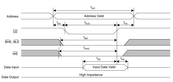
Figure 11. SRAM Write Cycle 2 (CE Controlled) <sup>[35, 36, 37, 38]</sup>
