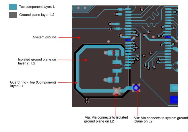
Figure 6. Recommended Layout for RTC
