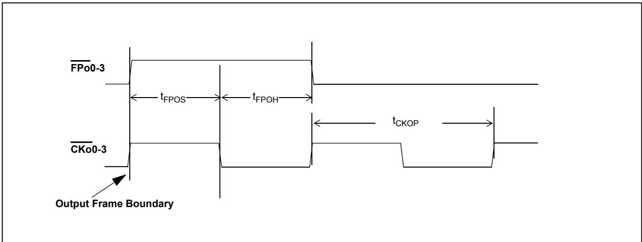
Figure 15 - GCI Frame Pulse and Clock Output Timing
