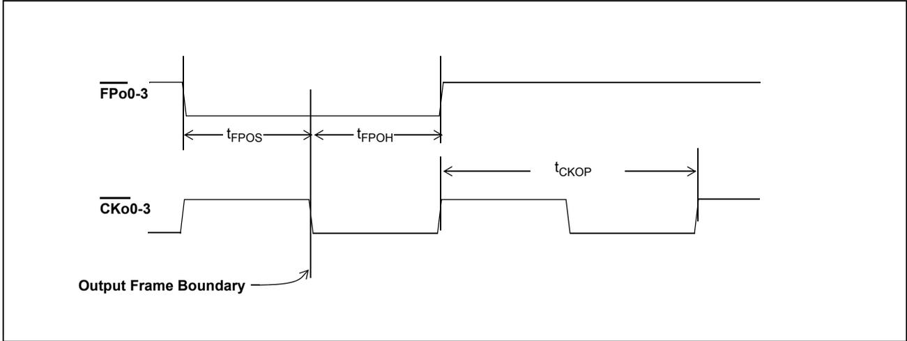
Figure 14 - ST-Bus Frame Pulse and Clock Output Timing
