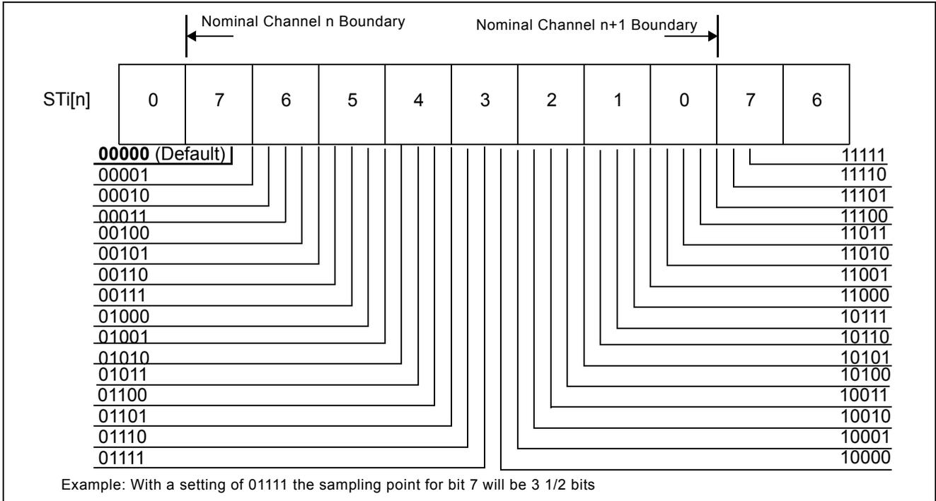
**Figure 5 - Input Sampling Point Delay Programming**
