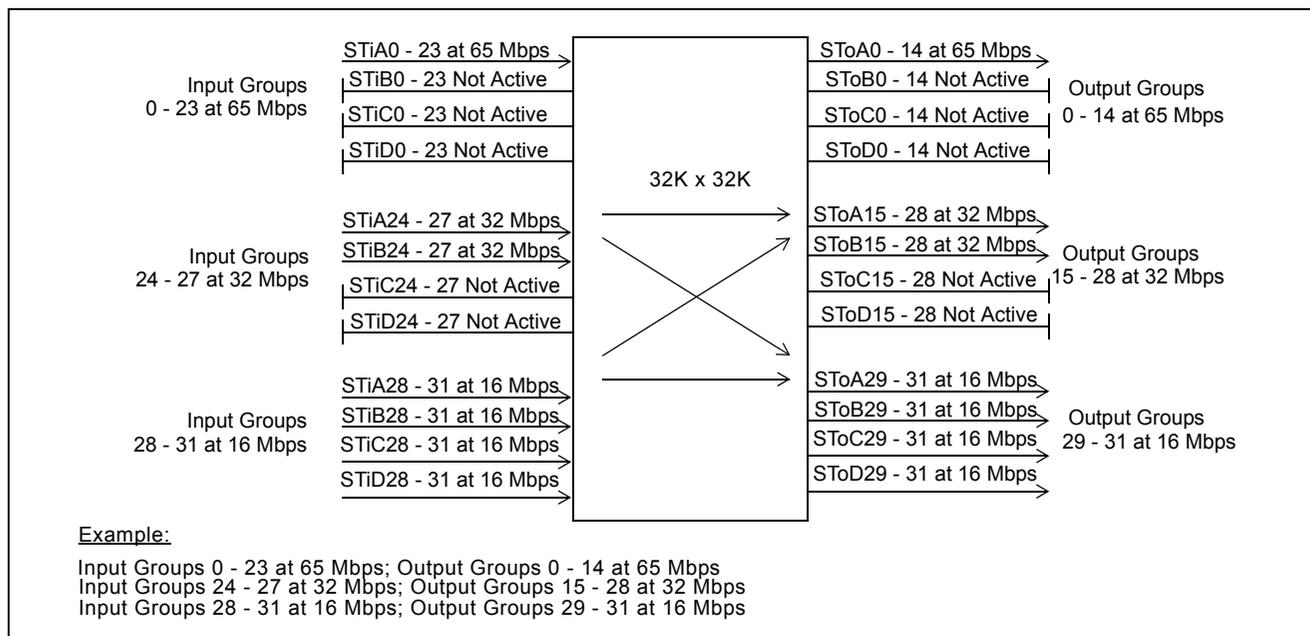
Figure 4 - Input and Output Data Rate Conversion Example
