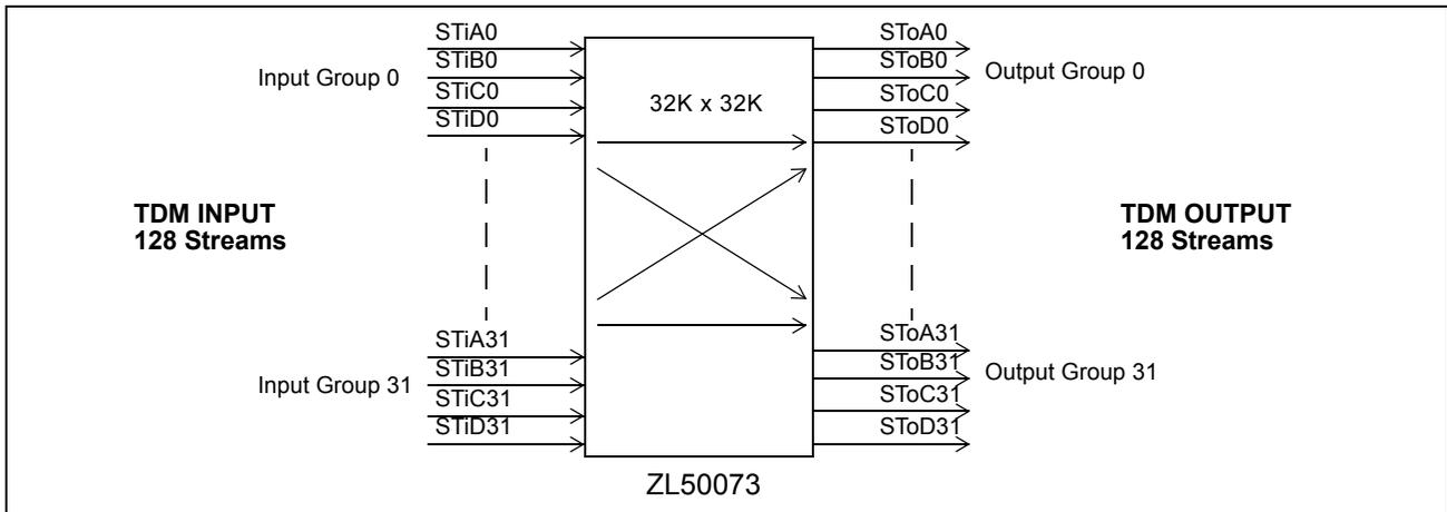
**Figure 2 - 32 K x 32 K Channel Basic Switch Configuration**
