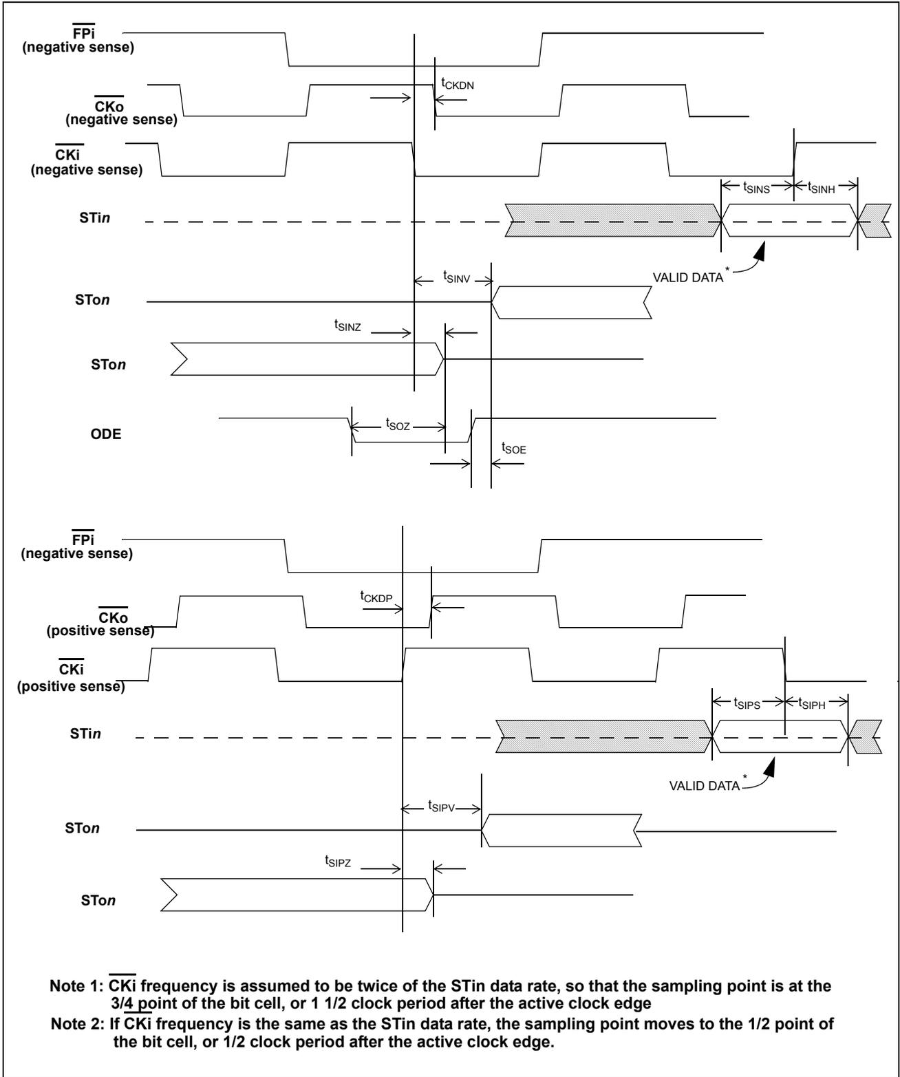
Figure 16 - Serial Data Timing to  $\overline{CKi}$
