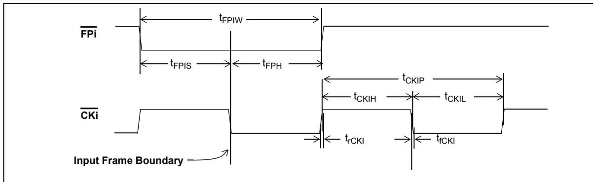
**Figure 12 - Frame Pulse Input and Clock Input**
