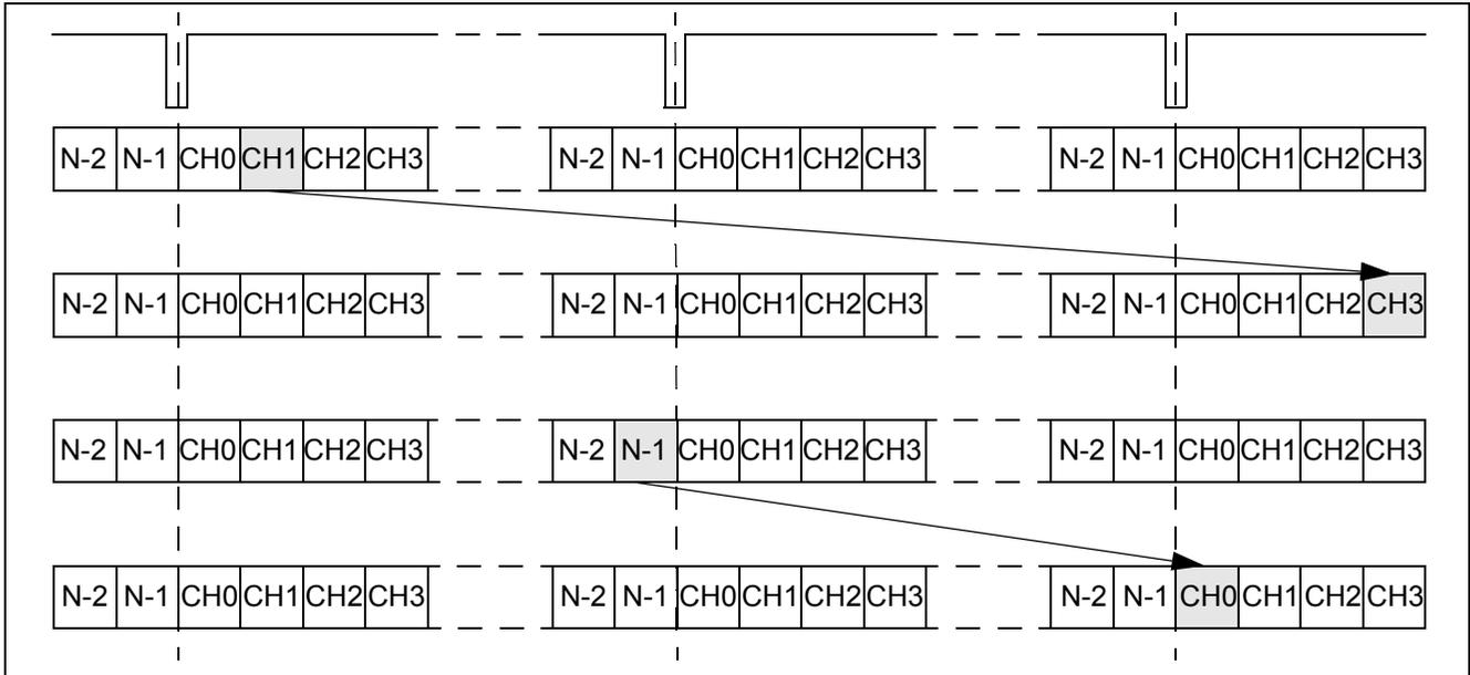
Figure 7 - Data Throughput Delay for Constant Delay
