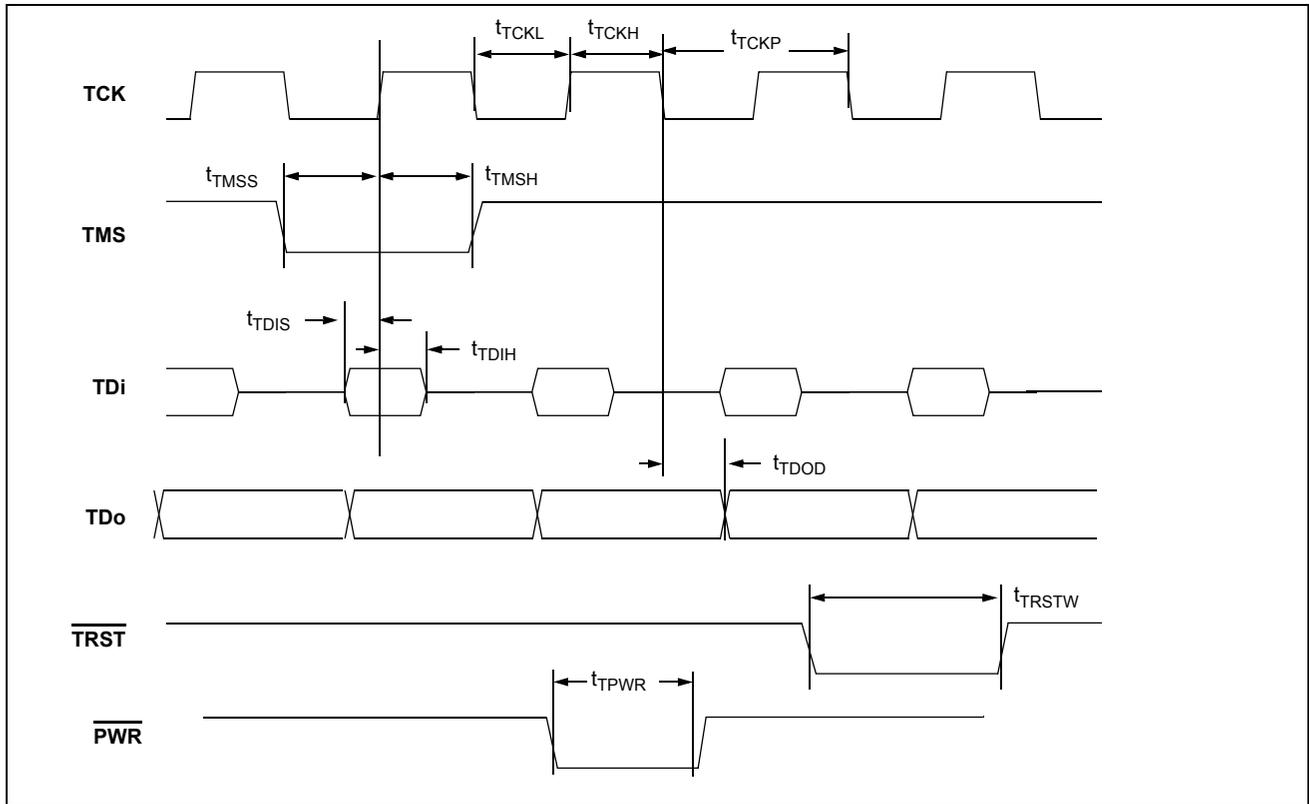
Figure 21 - IEEE 1149.1 Test Port &  $\overline{\text{PWR}}$  Reset Timing
