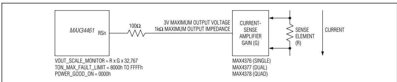
Figure 9. Current-Measuring Circuit
