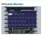
The "Parallel Monitor" function is also useful during actual operation for monitoring parallel input and output signals to and from the PV310.
