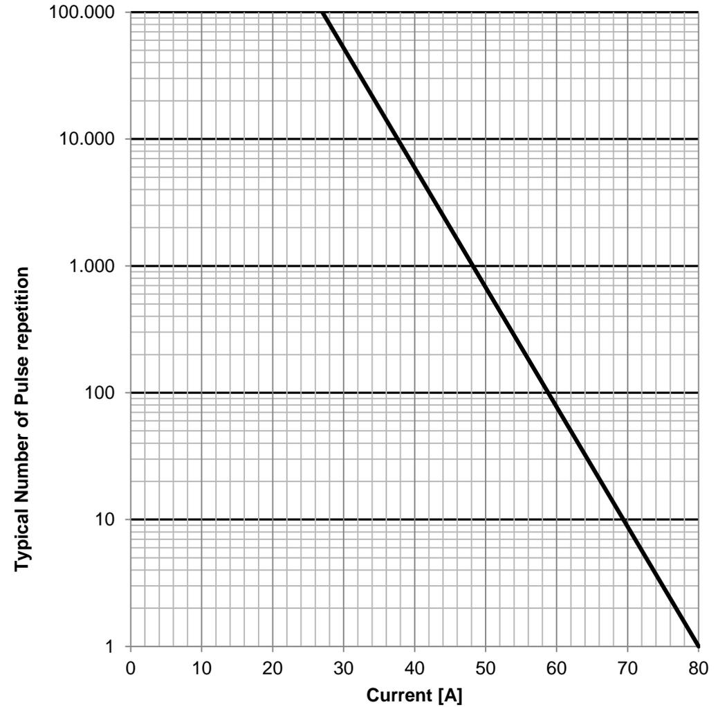
valid for ambient temperature: +25°C; 8 ms pulse length, 10 s break between pulse
