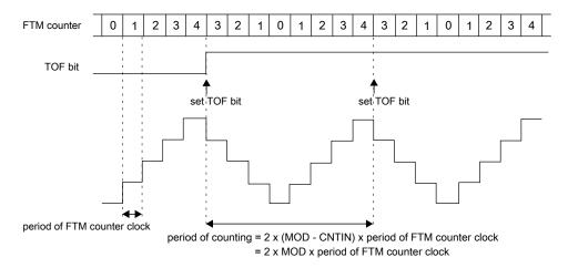
Figure 37-7. Example of up-down counting when CNTIN = 0x0000
