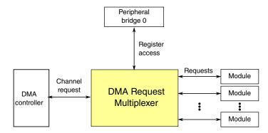
Figure 3-12. DMA request multiplexer configuration
