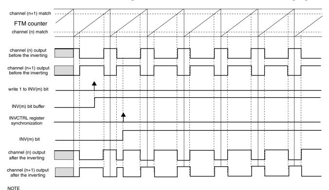
Figure 37-64. Channels (n) and (n+1) outputs after the inverting in Low-True (ELSnB:ELSnA = X:1) Combine mode
