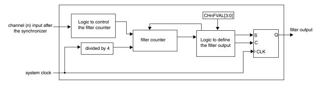
Figure 37-12. Channel input filter
