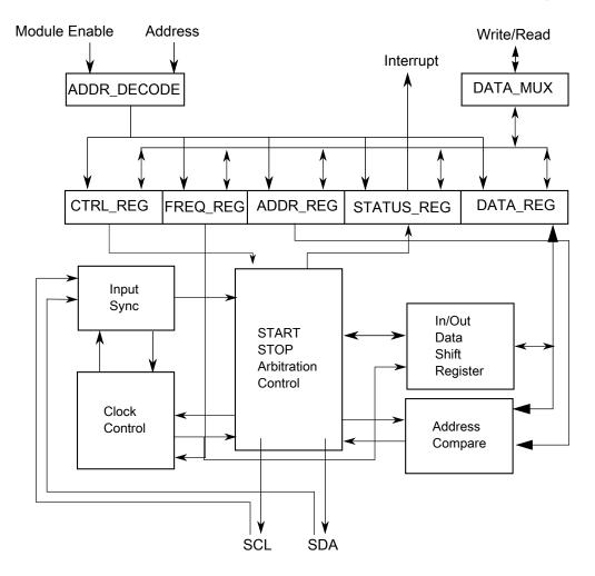
Figure 41-1. I2C Functional block diagram
