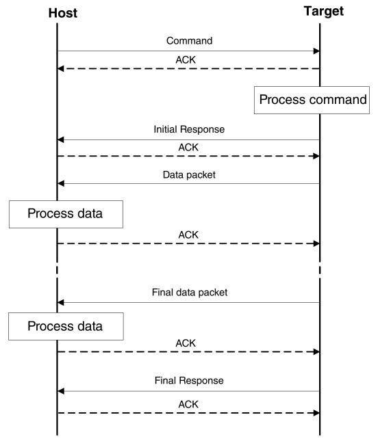
Figure 13-5. Command with outgoing data phase
