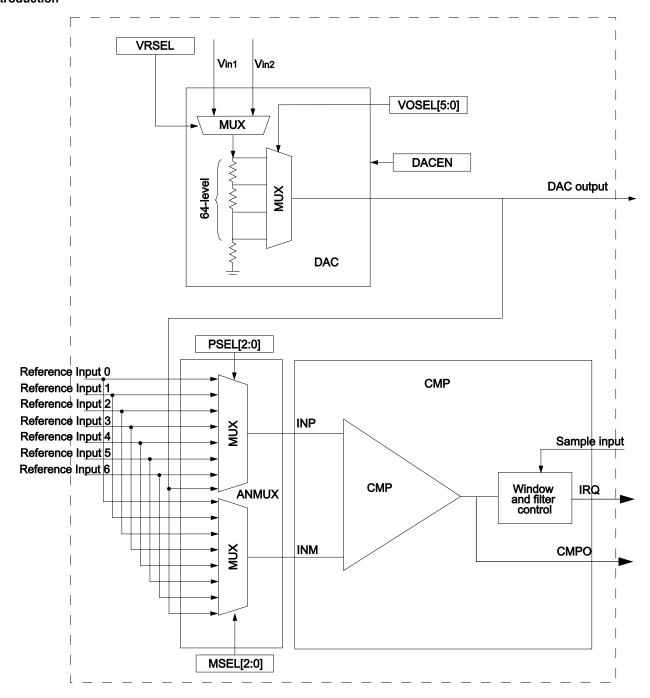
Figure 33-1. CMP, DAC and ANMUX block diagram
