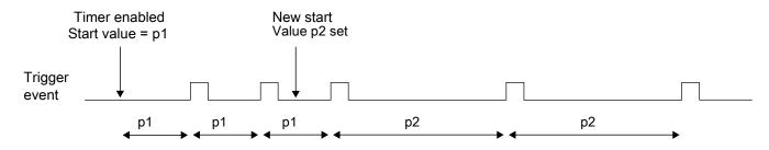
Figure 38-4. Dynamically setting a new load value
