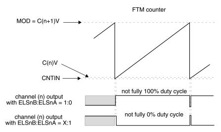
Figure 37-29. Channel (n) output if (CNTIN < C(n)V < MOD) and (C(n)V is Almost Equal to CNTIN) and (C(n+1)V = MOD)
