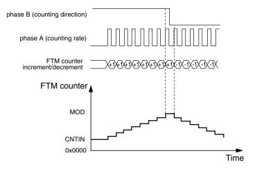
Figure 37-90. Quadrature Decoder – Count and Direction Encoding mode
