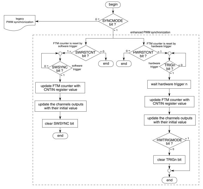
Figure 37-59. FTM counter synchronization flowchart
