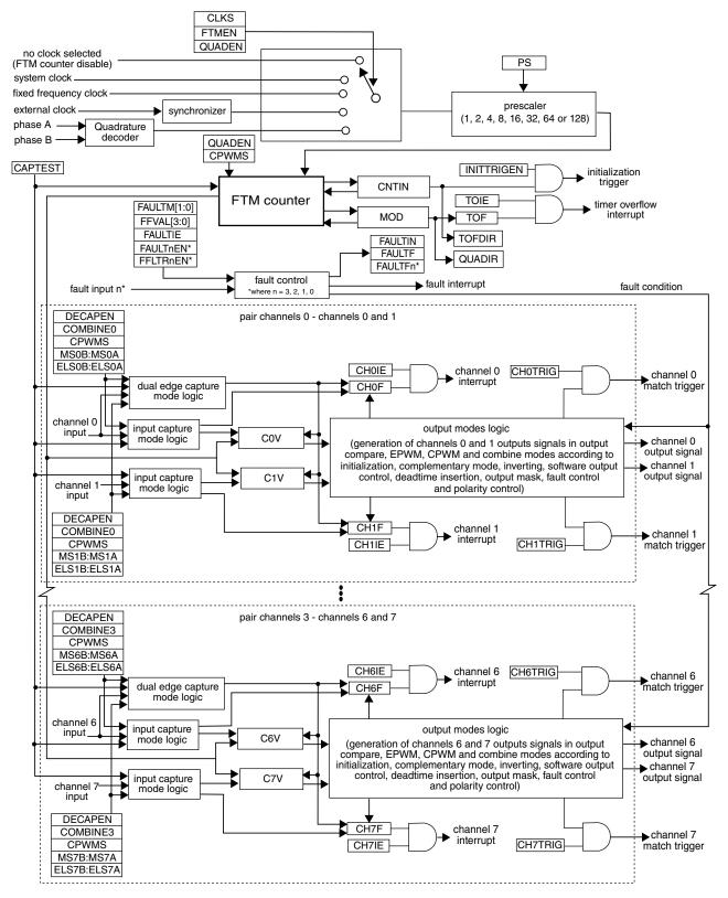
Figure 37-1. FTM block diagram
