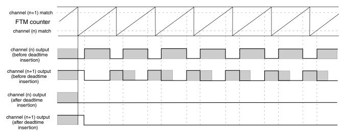
Figure 37-69. Example of the deadtime insertion (ELSnB:ELSnA = 1:0, POL(n) = 0, and POL(n+1) = 0) when the deadtime delay is comparable to channels (n) and (n+1) duty cycle
