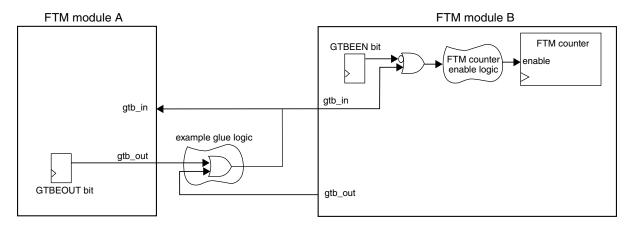
Figure 37-97. Global time base (GTB) block diagram
