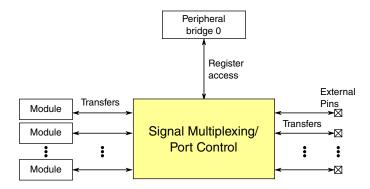
Figure 10-1. Signal multiplexing integration
