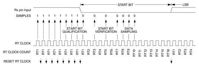
Figure 42-4. Receiver data sampling
