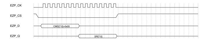
Figure 29-4. Read Status Register command sequence
