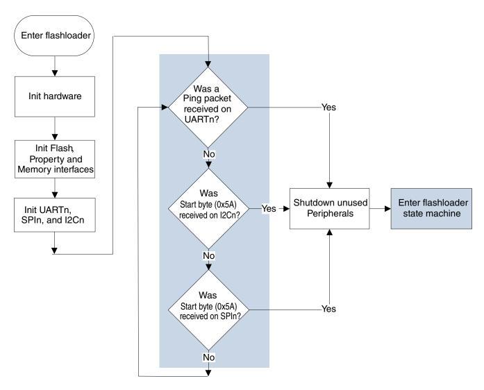
Figure 13-2. Kinetis Flashloader Start-up Flowchart
