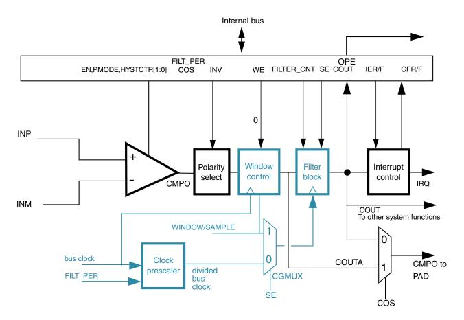
Figure 33-3. Comparator operation in Continuous mode
