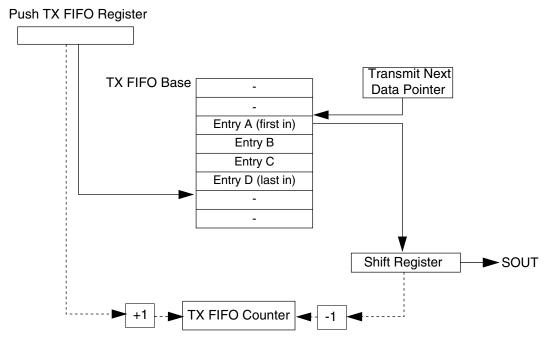
Figure 40-18. TX FIFO pointers and counter
