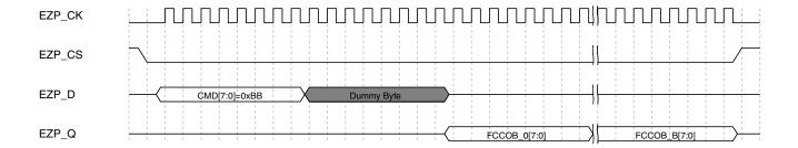
Figure 29-12. Read FCCOB Registers at High Speed command sequence
