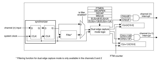
Figure 37-83. Dual Edge Capture mode block diagram
