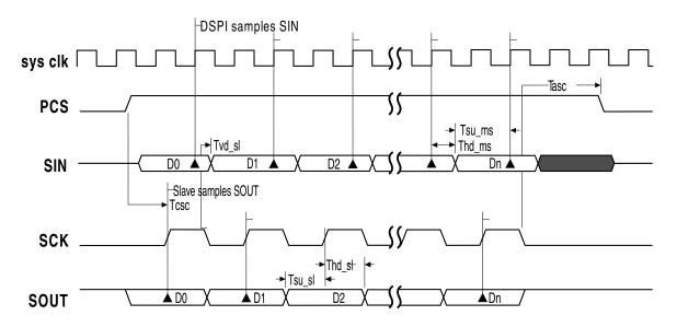
Figure 40-9. DSPI Modified Transfer Format (MTFE=1, CPHA=0,  $f_{sck} = f_{svs}/2$ )
