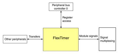
Figure 3-34. FlexTimer configuration
