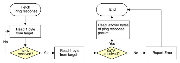
Figure 13-19. Host reads ping response from target via I2C
