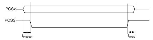
Figure 40-5. Peripheral Chip Select Strobe timing
