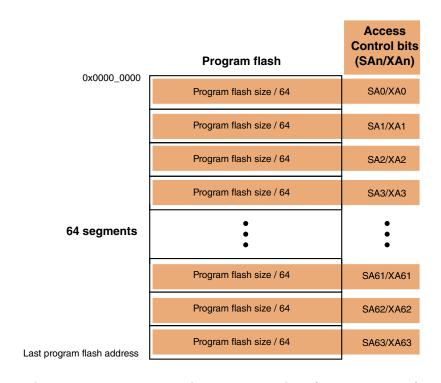
Figure 27-1. Program flash protection (64 segments)
