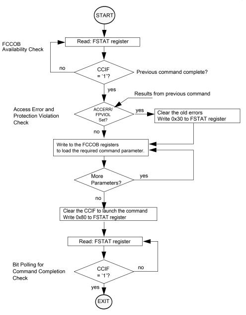
Figure 28-5. Generic flash command write sequence flowchart
