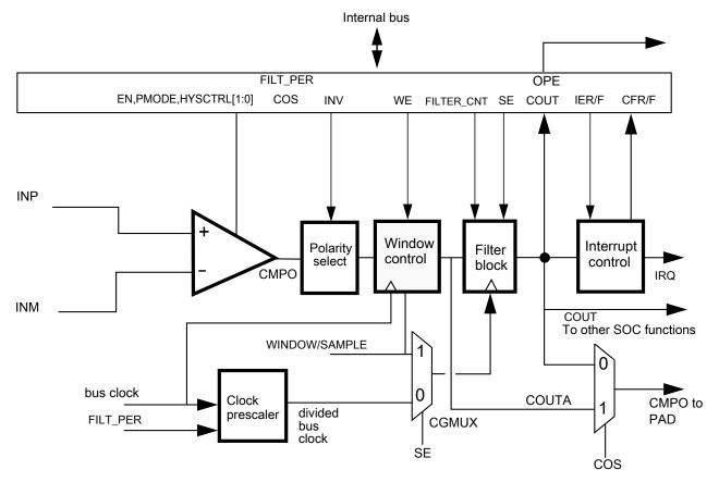
Figure 33-2. Comparator module block diagram
