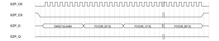
Figure 29-11. Write FCCOB Registers command sequence
