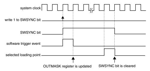
Figure 37-53. OUTMASK synchronization with (SYNCMODE = 0), (SYNCHOM = 1), (PWMSYNC = 0) and software trigger was used
