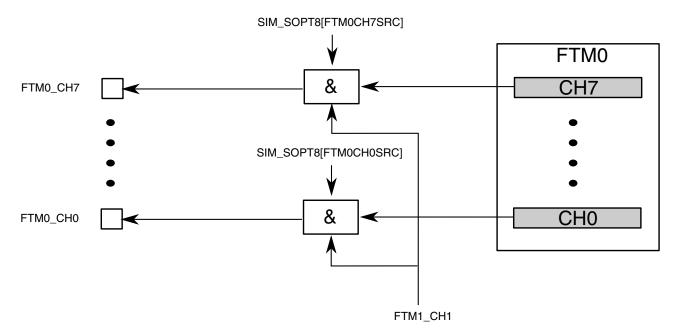
Figure 3-36. FTM Output Modulation
