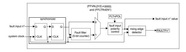
Figure 37-71. Fault input n control block diagram
