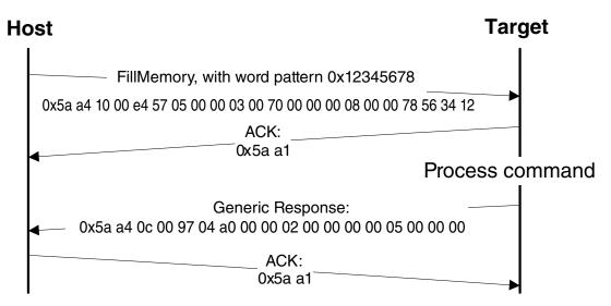
Figure 13-12. Protocol Sequence for FillMemory Command
