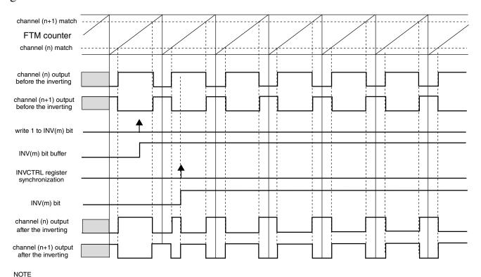
Figure 37-63. Channels (n) and (n+1) outputs after the inverting in High-True (ELSnB:ELSnA = 1:0) Combine mode
