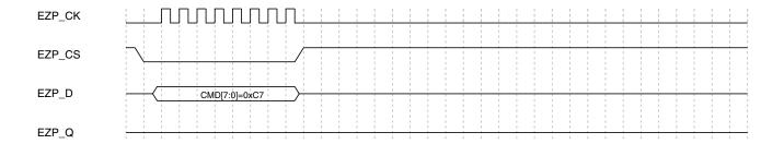
Figure 29-9. Bulk Erase command sequence
