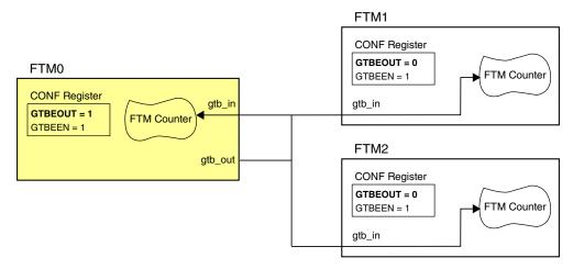
Figure 3-37. FTM Global Time Base Configuration
