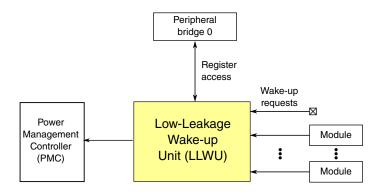
Figure 3-8. Low-Leakage Wake-up Unit configuration
