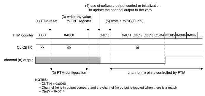
Figure 37-99. FTM behavior after reset when the channel (n) is in Output Compare mode
