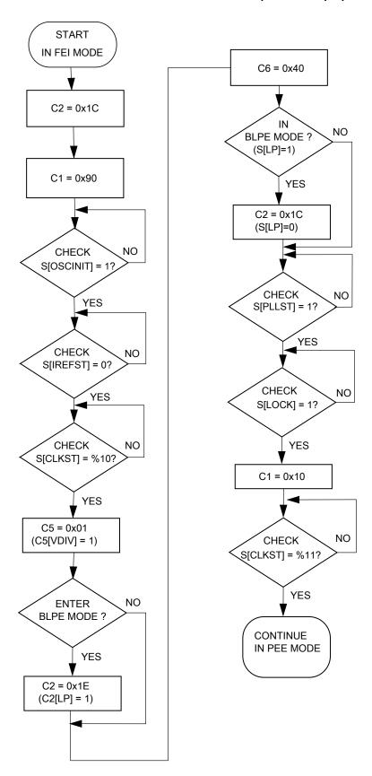
Figure 25-3. Flowchart of FEI to PEE mode transition using an 4 MHz crystal
