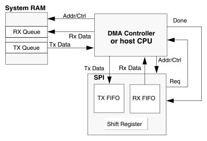
Figure 40-2. SPI with queues and DMA
