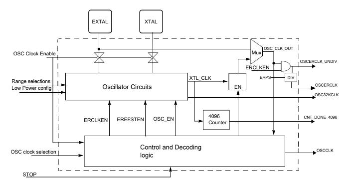
Figure 26-1. OSC Module Block Diagram
