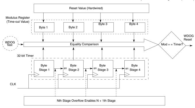
Figure 24-2. Watchdog timer byte splitting
