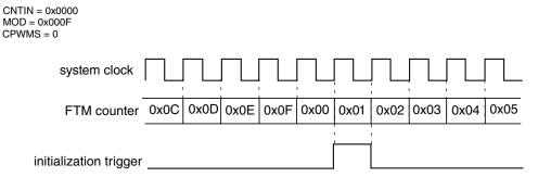
Figure 37-77. Initialization trigger is generated when the FTM counting achieves the CNTIN register value
