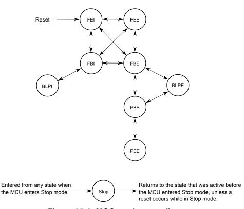
Figure 25-2. MCG mode state diagram
