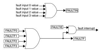
Figure 37-72. FAULTF and FAULTIN bits and fault interrupt
