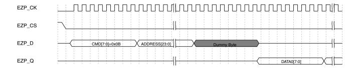
Figure 29-6. Read Data at High Speed command sequence
