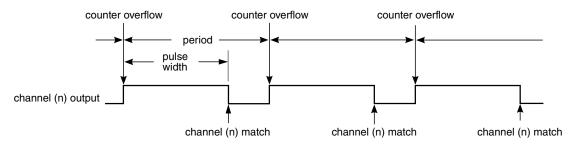
Figure 37-19. EPWM period and pulse width with ELSnB:ELSnA = 1:0
