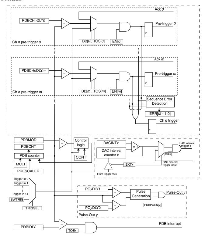
Figure 36-1. PDB block diagram
