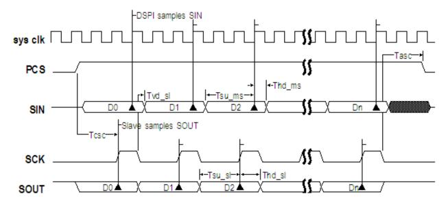
Figure 40-10. DSPI Modified Transfer Format (MTFE=1, CPHA=0,  $f_{sck} = f_{sys}/3$ )
