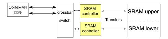
Figure 3-21. SRAM configuration
