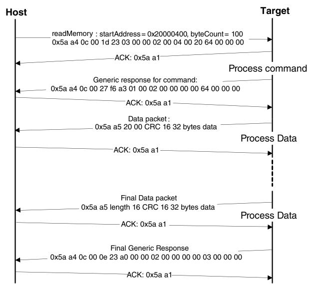
Figure 13-17. Command sequence for read memory
