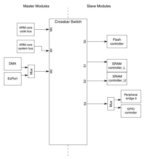
Figure 3-10. Crossbar-Light switch integration
