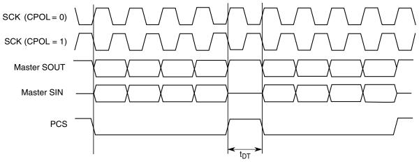
Figure 40-16. Continuous SCK Timing Diagram (CONT=0)
