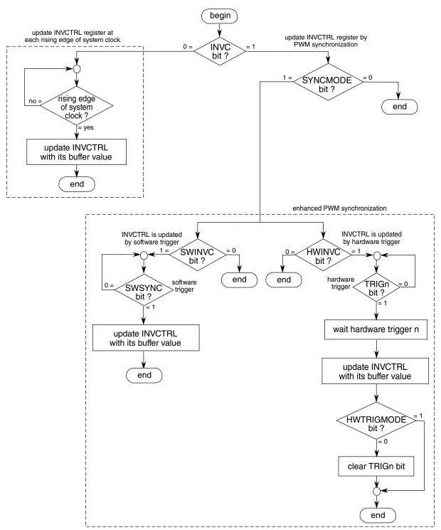
Figure 37-56. INVCTRL register synchronization flowchart
