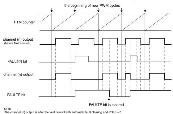
Figure 37-73. Fault control with automatic fault clearing
