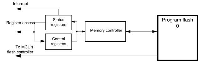
Figure 28-1. Flash Block Diagram
