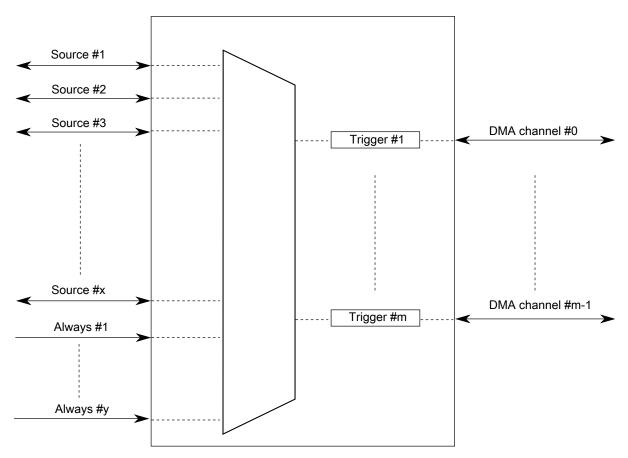
Figure 21-2. DMAMUX triggered channels
