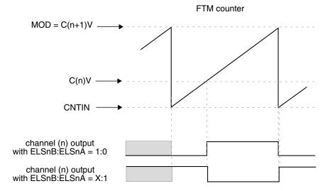
Figure 37-27. Channel (n) output if (CNTIN < C(n)V < MOD) and (C(n+1)V = MOD)
