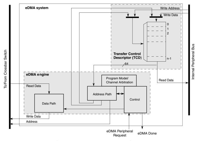
Figure 22-1. eDMA system block diagram
