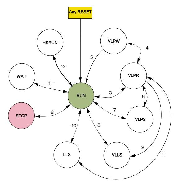
Figure 15-1. Power mode state diagram
