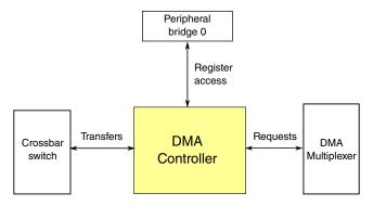
Figure 3-13. DMA Controller configuration
