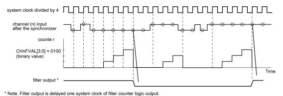
Figure 37-13. Channel input filter example
