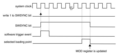
Figure 37-47. MOD synchronization with (SYNCMODE = 0), (PWMSYNC = 0), (REINIT = 0), and software trigger was used
