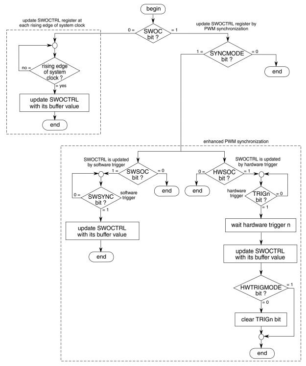
Figure 37-57. SWOCTRL register synchronization flowchart
