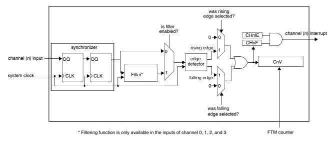
Figure 37-11. Input Capture mode
