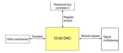
Figure 3-30. 12-bit DAC configuration
