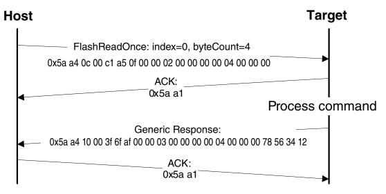
Figure 13-14. Protocol Sequence for FlashReadOnce Command
