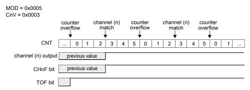
Figure 37-18. Example of the Output Compare mode when the match sets the channel output
