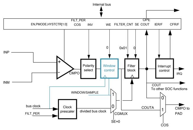
Figure 33-5. Sampled, Non-Filtered (# 3B): sampling interval internally derived
