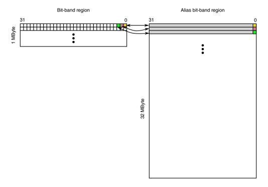
Figure 4-1. Alias bit-band mapping
