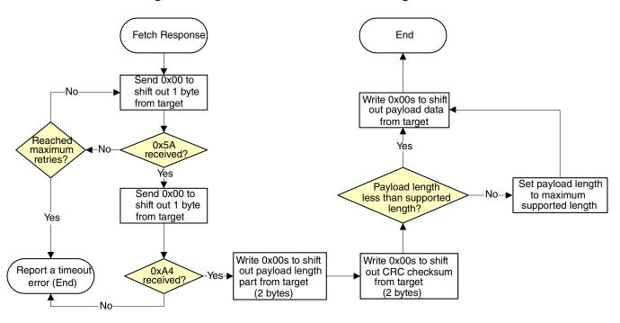
Figure 13-24. Host reads response from target via SPI
