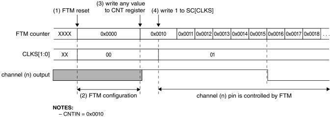
Figure 37-98. FTM behavior after reset when the channel (n) is in Combine mode
