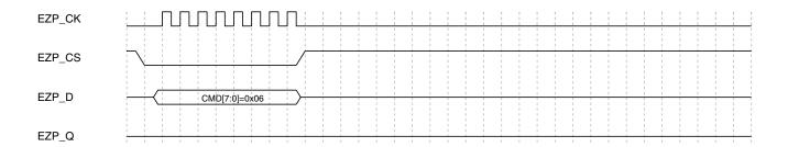
Figure 29-2. Write Enable command sequence
