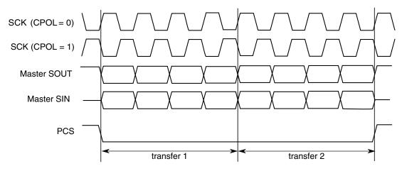
Figure 40-17. Continuous SCK timing diagram (CONT=1)
