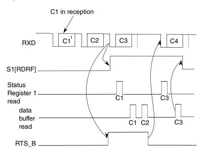
Figure 42-11. Receiver hardware flow control timing diagram
