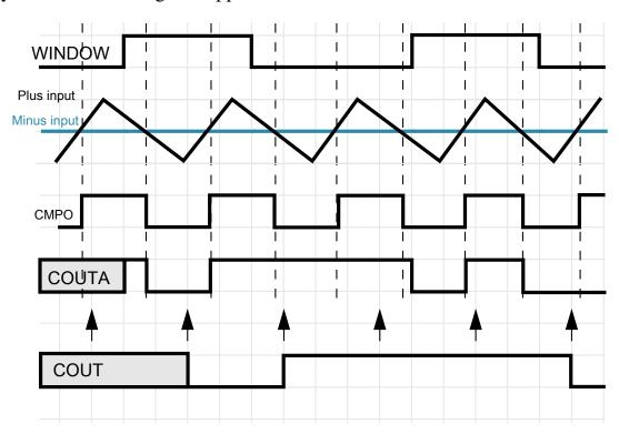
Figure 33-10. Windowed/resampled mode operation
