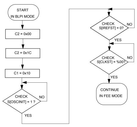
Figure 25-5. Flowchart of BLPI to FEE mode transition using an 4 MHz crystal
