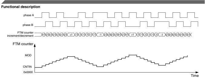
Figure 37-91. Quadrature Decoder – Phase A and Phase B Encoding mode
