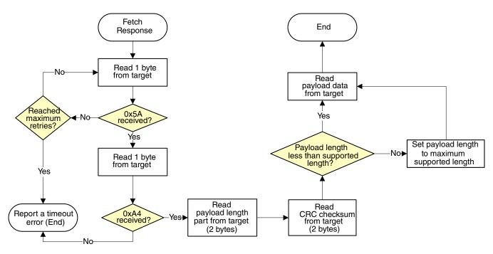
Figure 13-21. Host reads response from target via I2C
