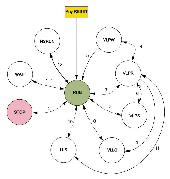
Figure 7-1. Power mode state transition diagram
