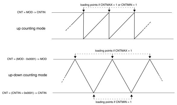
Figure 37-45. Boundary cycles and loading points
