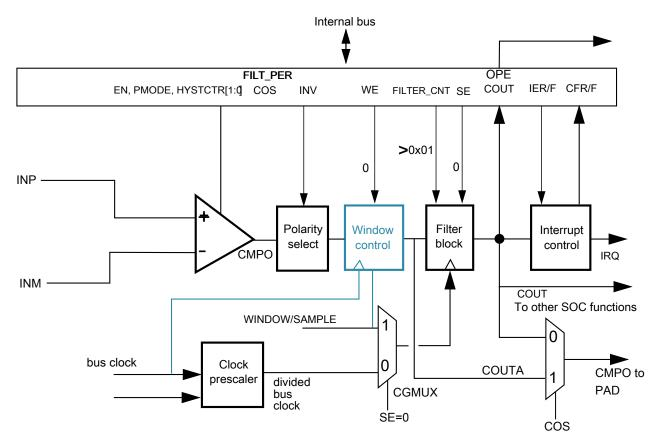
Figure 33-7. Sampled, Filtered (# 4B): sampling point internally derived
