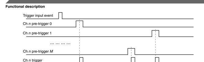
Figure 36-2. Pre-trigger and trigger outputs
