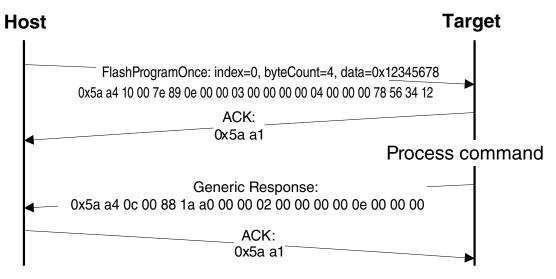
Figure 13-13. Protocol Sequence for FlashProgramOnce Command
