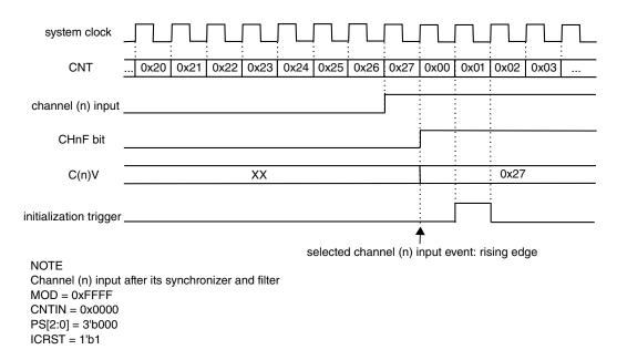
Figure 37-81. Initialization trigger is generated if the channel (n) is in Input Capture mode, ICRST = 1 and the selected input capture event occurs in the channel (n) input
