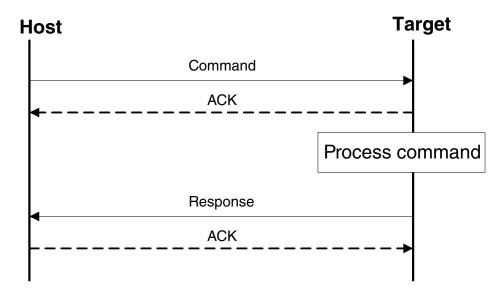
Figure 13-3. Command with No Data Phase
