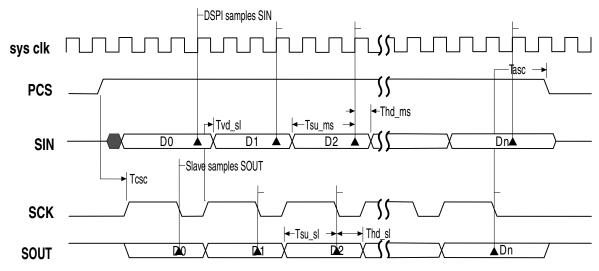
Figure 40-12. DSPI Modified Transfer Format (MTFE=1, CPHA=1,  $f_{sck} = f_{svs}/3$ )
