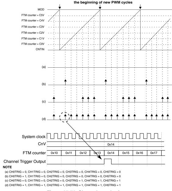
Figure 37-76. Channel match trigger
