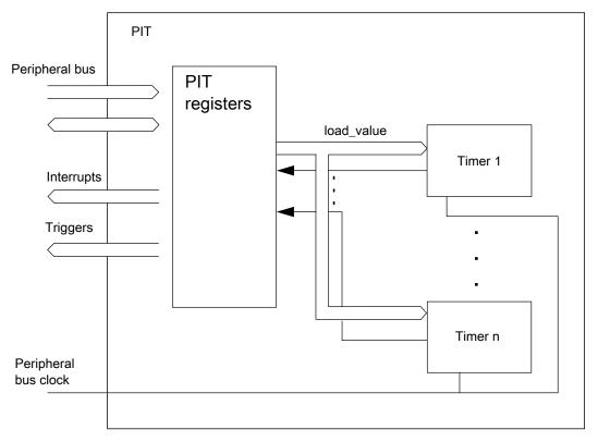
Figure 38-1. Block diagram of the PIT
