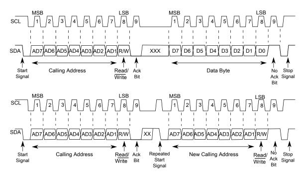
Figure 41-2. I2C bus transmission signals
