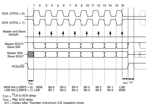
Figure 40-7. Module transfer timing diagram (MTFE=0, CPHA=1, FMSZ=8)
