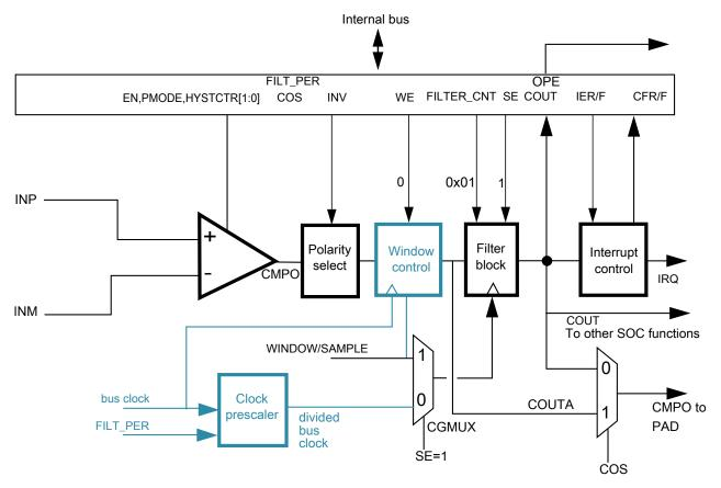
Figure 33-4. Sampled, Non-Filtered (# 3A): sampling point externally driven
