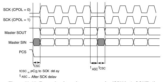
Figure 40-15. Example of continuous transfer (CPHA=1, CONT=1)
