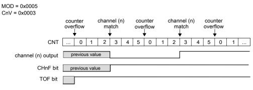
Figure 37-16. Example of the Output Compare mode when the match toggles the channel output
