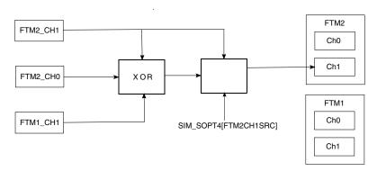
Figure 3-35. FTM Hall Sensor Configuration
