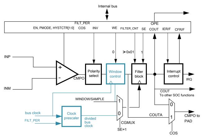
Figure 33-6. Sampled, Filtered (# 4A): sampling point externally driven
