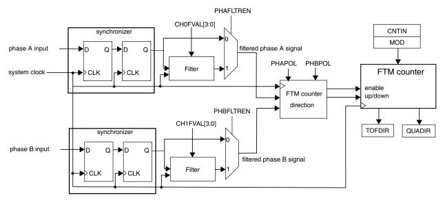
Figure 37-89. Quadrature Decoder block diagram
