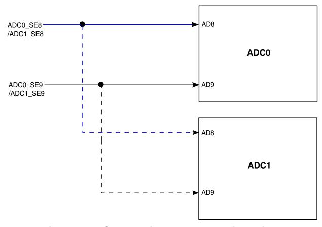
Figure 3-28. ADC hardware interleaved channels integration
