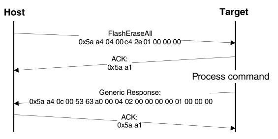
Figure 13-10. Protocol Sequence for FlashEraseAll Command
