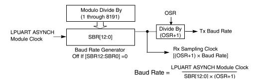
Figure 43-3. LPUART baud rate generation
