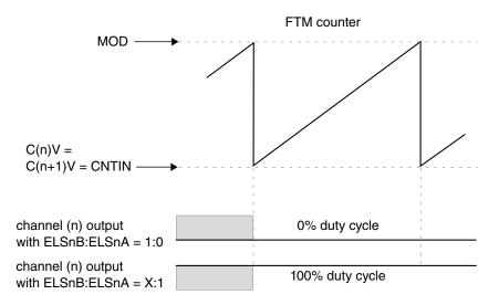
Figure 37-33. Channel (n) output if (C(n)V = C(n+1)V = CNTIN)
