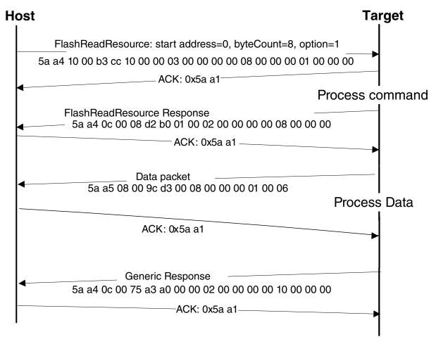
Figure 13-15. Protocol Sequence for FlashReadResource Command
