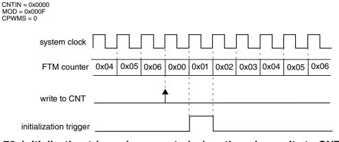
Figure 37-78. Initialization trigger is generated when there is a write to CNT register
