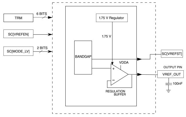
Figure 35-1. Voltage reference block diagram
