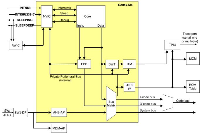
Figure 9-1. Cortex-M4 Debug Topology
