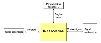
Figure 3-26. 16-bit SAR ADC configuration
