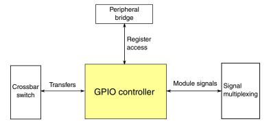
Figure 3-44. GPIO configuration
