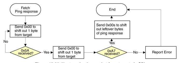
Figure 13-22. Host reads ping packet from target via SPI
