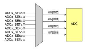
Figure 3-27. ADCx\_SEn channels a and b selection
