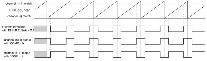
Figure 37-42. Channel (n+1) output in Complementary mode with (ELSnB:ELSnA = X:1)
