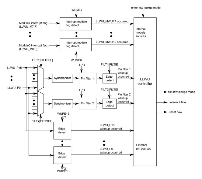
Figure 17-1. LLWU block diagram
