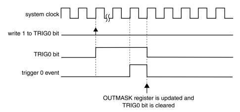
Figure 37-54. OUTMASK synchronization with (SYNCMODE = 0), (HWTRIGMODE = 0), (SYNCHOM = 1), (PWMSYNC = 0), and a hardware trigger was used
