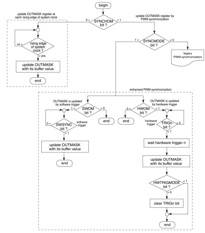
Figure 37-52. OUTMASK register synchronization flowchart
