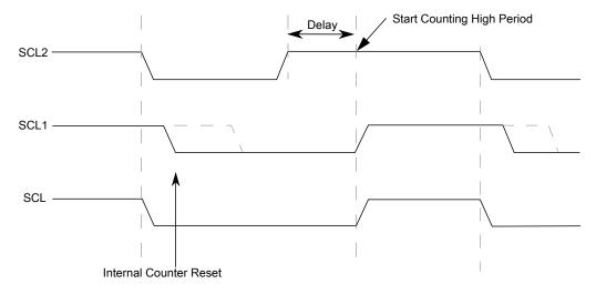
Figure 41-3. I2C clock synchronization
