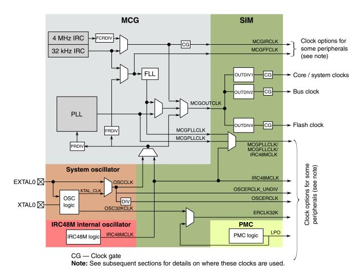
Figure 5-1. Clocking diagram
