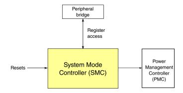
Figure 3-7. System Mode Controller configuration
