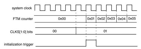
Figure 37-80. Initialization trigger is generated if (CNT = CNTIN), (CLKS[1:0] = 0:0), and a value different from zero is written to CLKS[1:0] bits
