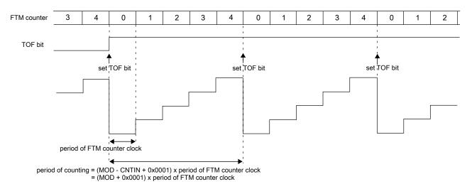
Figure 37-5. Example of FTM up counting with CNTIN = 0x0000
