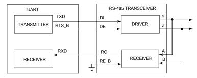
Figure 42-29. Transceiver driver enable using RTS
