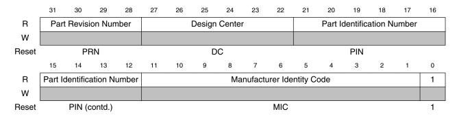
The following table describes the device identification register functions.
