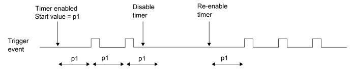
Figure 38-2. Stopping and starting a timer
