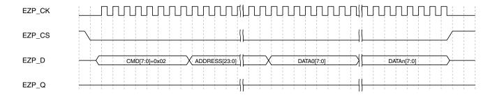
Figure 29-7. Section Program command sequence
