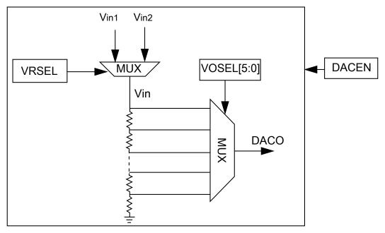
Figure 33-12. 6-bit DAC block diagram
