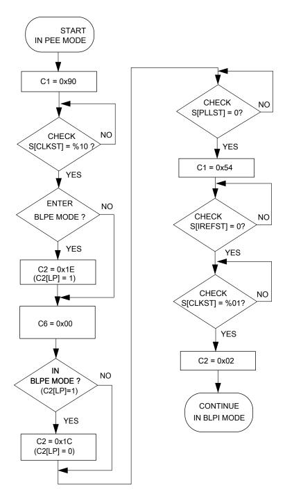
Figure 25-4. Flowchart of PEE to BLPI mode transition using an 4 MHz crystal
