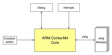
Figure 3-1. Core configuration
