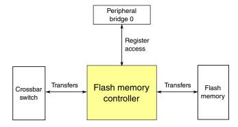
Figure 3-20. Flash memory controller configuration
