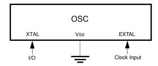
Figure 26-5. External Clock Connections
