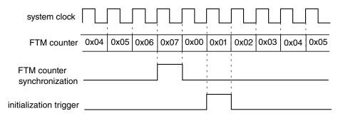
Figure 37-79. Initialization trigger is generated when there is the FTM counter synchronization
