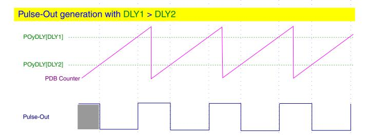
Figure 36-3. How Pulse Out is generated
