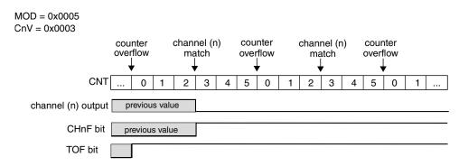
Figure 37-17. Example of the Output Compare mode when the match clears the channel output
