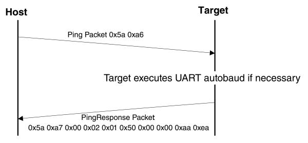
Figure 13-6. Ping Packet Protocol Sequence
