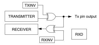
Figure 42-25. Loop operation (C1[LOOPS] = 1, C1[RSRC] = 0)
