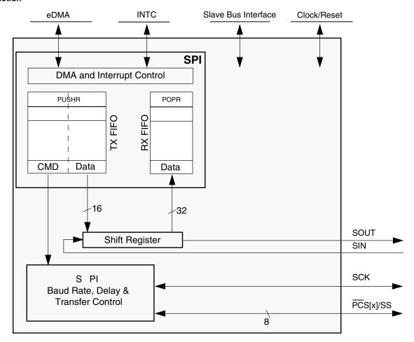
Figure 40-1. SPI Block Diagram
