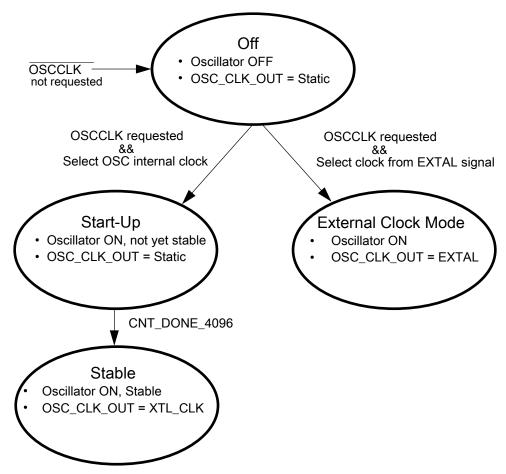
Figure 26-6. OSC Module state diagram
