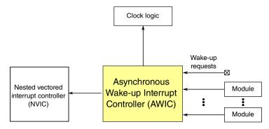
Figure 3-3. Asynchronous Wake-up Interrupt Controller configuration
