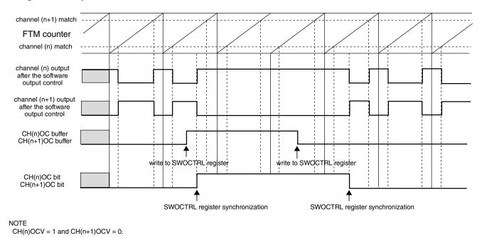
Figure 37-65. Example of software output control in Combine and Complementary mode
