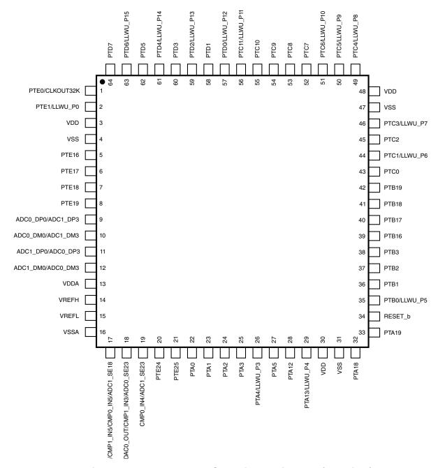
Figure 10-2. KV31F 64 LQFP pinout diagram (top view)
