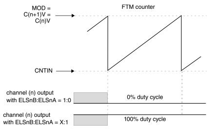
Figure 37-34. Channel (n) output if (C(n)V = C(n+1)V = MOD)
