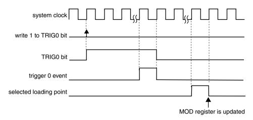
Figure 37-48. MOD synchronization with (SYNCMODE = 0), (HWTRIGMODE = 0), (PWMSYNC = 0), (REINIT = 0), and a hardware trigger was used
