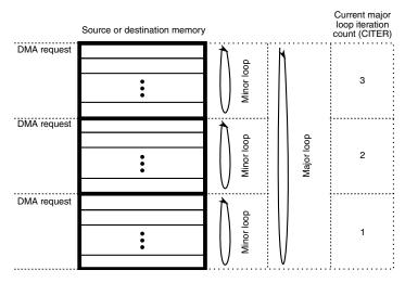
Figure 22-5. Example of multiple loop iterations
