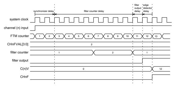
Figure 37-14. Input capture example
