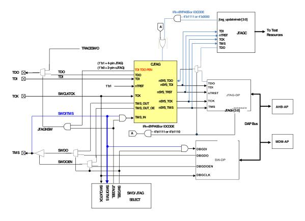
Figure 9-2. Modified Debug Port
