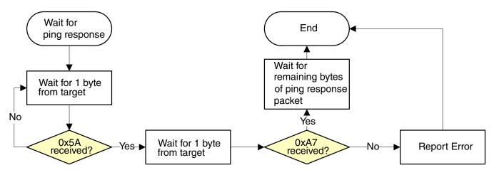
Figure 13-26. Host reads a ping response from target via UART
