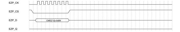
Figure 29-10. Reset Chip command sequence
