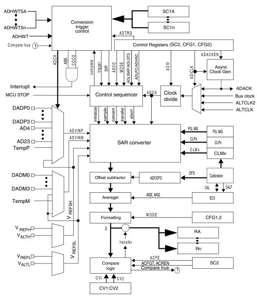
Figure 32-1. ADC block diagram
