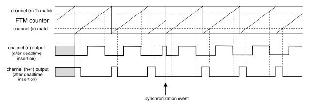
Figure 37-58. FTM counter synchronization
