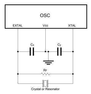
Figure 26-4. Crystal/Ceramic Resonator Connections - Connection 3
