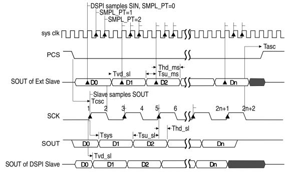
Figure 40-8. DSPI Modified Transfer Format (MTFE=1, CPHA=0,  $f_{sck} = f_{svs}/4$ )
