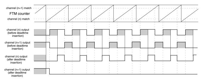
Figure 37-68. Example of the deadtime insertion (ELSnB:ELSnA = 1:0, POL(n) = 0, and POL(n+1) = 0) when the deadtime delay is comparable to channel (n+1) duty cycle
