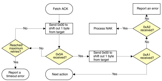
Figure 13-23. Host reads ACK from target via SPI
