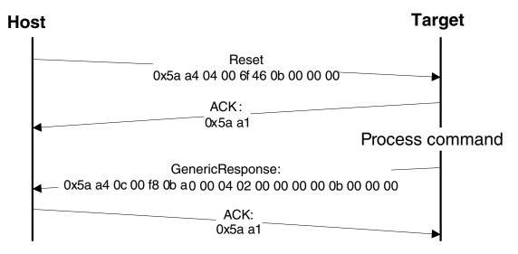
Figure 13-18. Protocol Sequence for Reset Command
