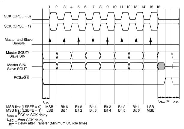
Figure 40-6. Module transfer timing diagram (MTFE=0, CPHA=0, FMSZ=8)
