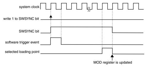
Figure 37-51. MOD synchronization with (SYNCMODE = 0) and (PWMSYNC = 1)
