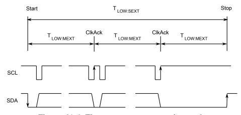
Figure 41-4. Timeout measurement intervals
