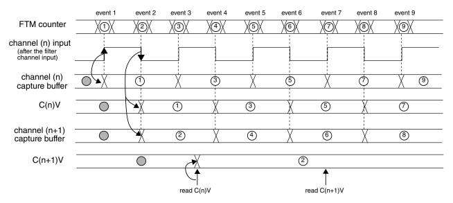
Figure 37-88. Dual Edge Capture mode read coherency mechanism
