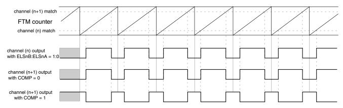
Figure 37-41. Channel (n+1) output in Complementary mode with (ELSnB:ELSnA = 1:0)
