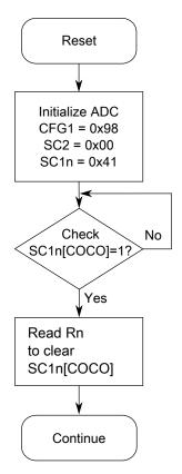
Figure 32-2. Initialization flowchart example
