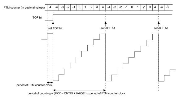
Figure 37-4. Example of FTM up and signed counting
