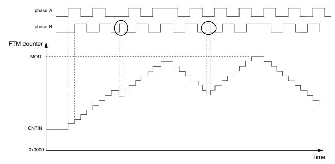
Figure 37-94. Motor position jittering in a mid count value
