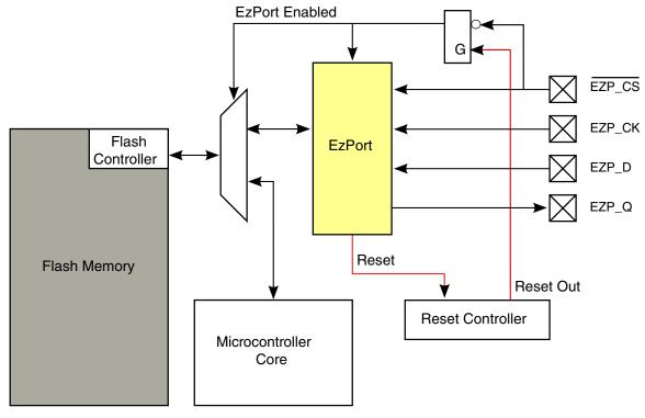
Figure 29-1. EzPort block diagram
