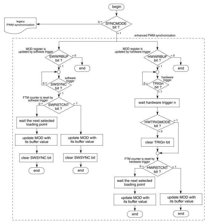
Figure 37-46. MOD register synchronization flowchart
