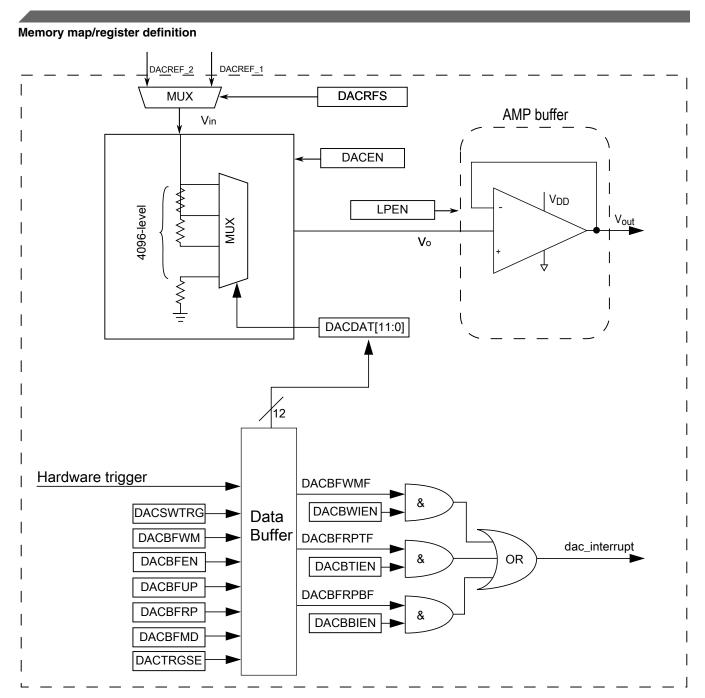
Figure 34-1. DAC block diagram
