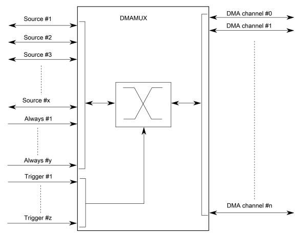
Figure 21-1. DMAMUX block diagram
