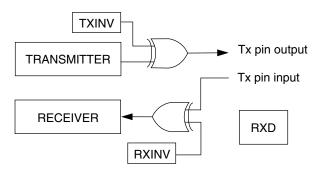
Figure 42-24. Single-wire operation (C1[LOOPS] = 1, C1[RSRC] = 1)
