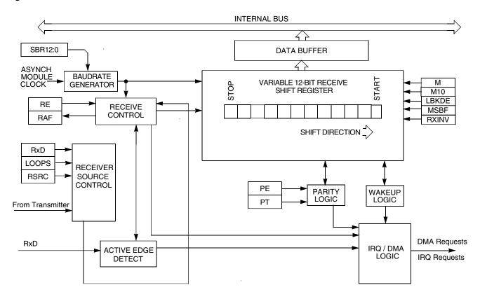
Figure 43-2. LPUART receiver block diagram
