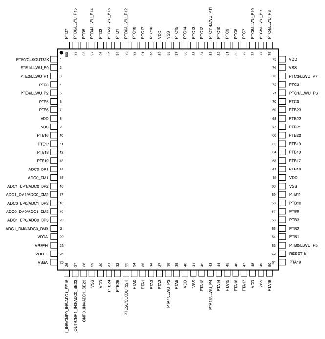
Figure 10-3. KV31F 100 LQFP pinout diagram (top view)
