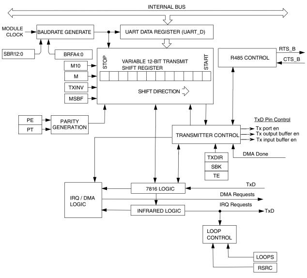
Figure 42-1. Transmitter Block Diagram
