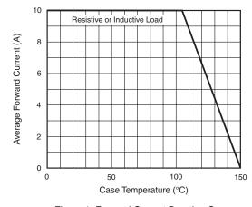
Figure 1. Forward Current Derating Curve
