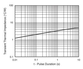
Figure 5. Typical Transient Thermal Impedance Per Diode
