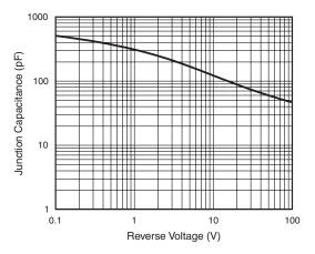
Figure 6. Typical Junction Capacitance Per Diode
