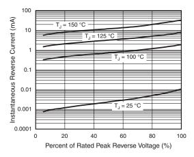
Figure 4. Typical Reverse Characteristics Per Diode
