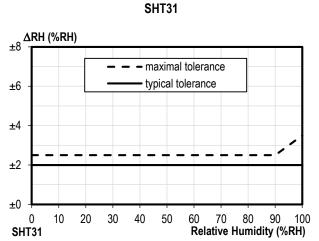
Figure 3 Tolerance of RH at 25°C for SHT31
