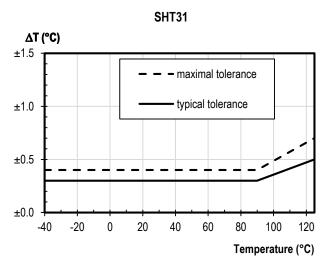
Figure 7 Temperature accuracy of the SHT31 sensor.
