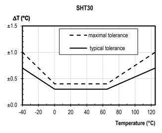
Figure 6 Temperature accuracy of the SHT30 sensor.
