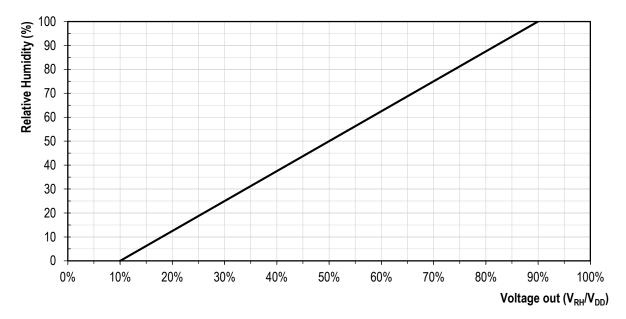
Figure 9 Relationship between the ratiometric analog voltage output and the measured relative humidity.
