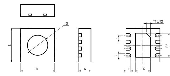
Figure 12 Dimensional drawing of SHT3x-ARP sensor package.
