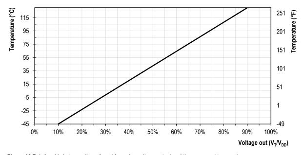
Figure 10 Relationship between the ratiometric analog voltage output and the measured temperature
