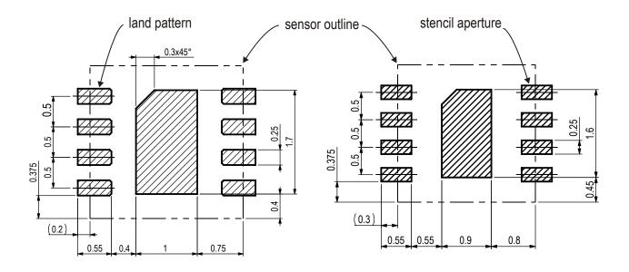
**Figure 13** Recommended metal land pattern (left) and stencil apertures (right) for the SHT3x-ARP. The dashed lines represent the outer dimension of the DFN package. The PCB pads (left) and stencil apertures (right) are indicated through the shaded areas.
