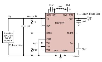
15V Converter Powered from Flexible Solar Panel
