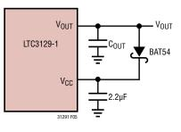
Figure 5. Example of  $V_{\mbox{CC}}$  Bootstrap
