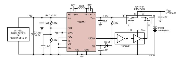
Solar Powered Converter Extends Battery Life in Low Power 3V Primary Battery Applications
