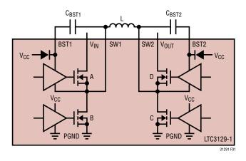
Figure 1. Power Stage Schematic
