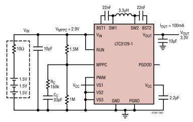
NOTE:  $R_C$  and  $C_C$  have been added for improved MPPC loop stability when using an input capacitor value less than the recommended minimum of  $22\mu F$
