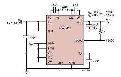
Low Noise, Fixed Frequency, Wide V<sub>IN</sub> Range 12V Converter
