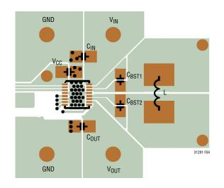
Figure 4. Typical 2-Layer PC Board Layout (MSE Package)
