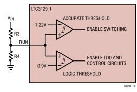
Figure 2. Accurate RUN Pin Comparator
